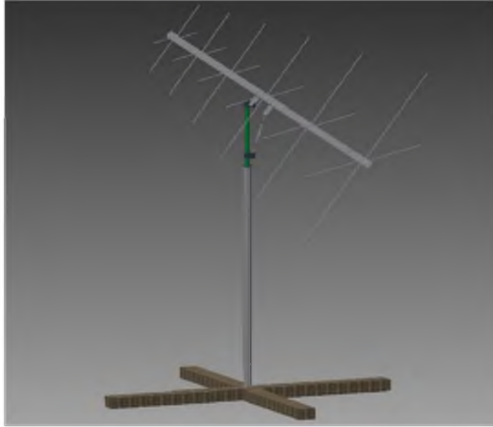
Figure 3.11: Dual polarized TARA Log Periodic Dipole Antenna (LPDA).
