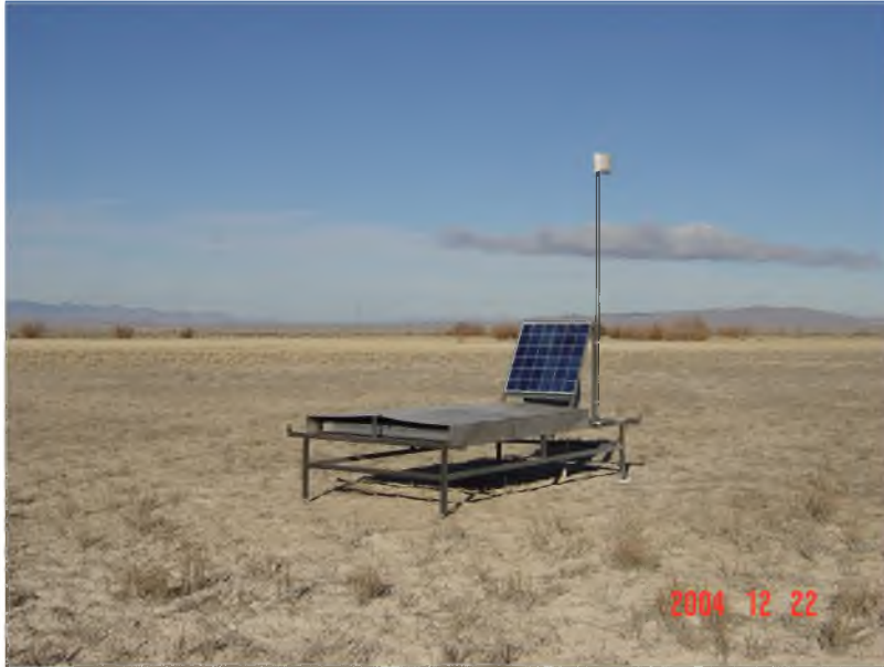
Figure 1.10: Picture of a single Telescope Array surface detector (SD), composed of a communications tower, solar panel for providing power to electronics and plastic scintillator enclosed in sheet metal.
