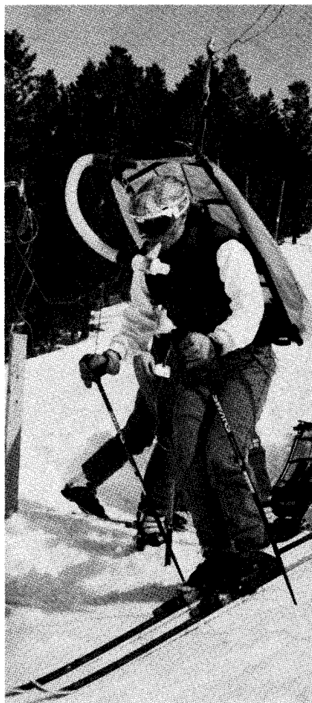
A test participant prepares to run a course with an apparatus designed to capture expired air in a Douglas bag.
