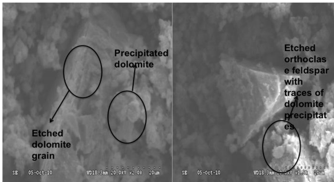
Figure 3- 29: Traces of dolomite precipitates in reacted sample after 4 weeks
