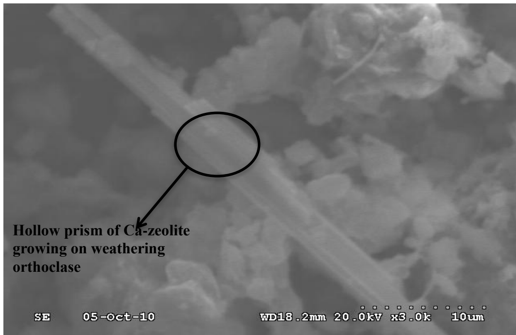
Figure 3- 27: Hollow prism of calcium zeolite 3 weeks after the start of the experiment
