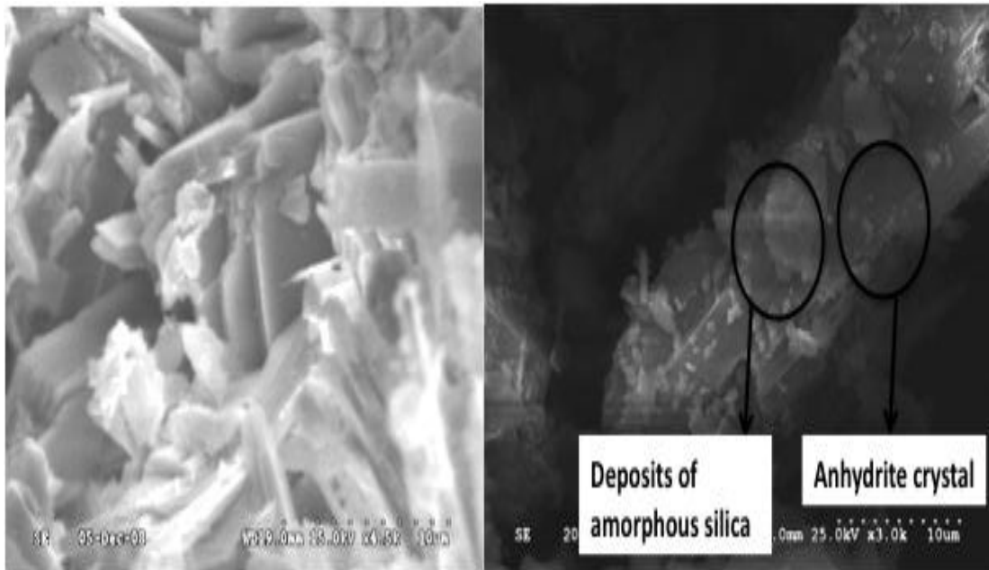
Figure 3- 37: Growth of anhydrite crystals after 37 days, and anhydrite + amorphous silica (right)
