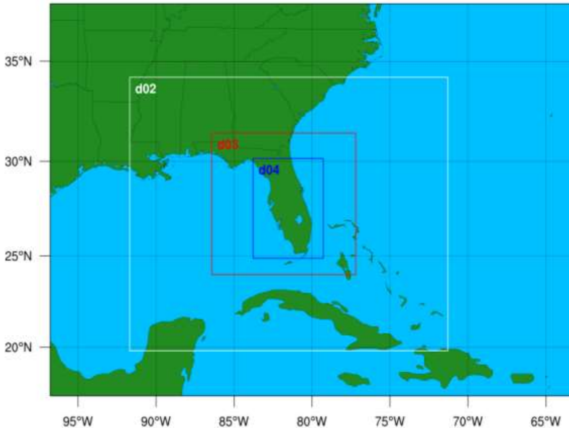
Figure 2.5 WRF simulation domains for the 27-km grid (d01 – color map), 9-km grid (d02 – white box), 3-km grid (d03 – red box), and 1-km grid (d04 – blue box).
