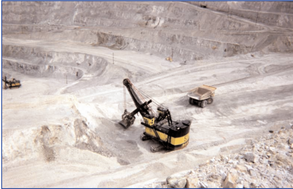
Kennecott's Bingham Canyon mine, Bingham mining district. The electric shovel has a 98-ton rock capacity scoop. The haulage truck holds 255 to 360 tons of rock.
