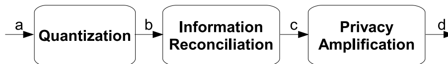
Figure 2.1. Secret key extraction process. a - RSS measurements, b - quantized bits, c - reconciled bits, d - secret bits.
