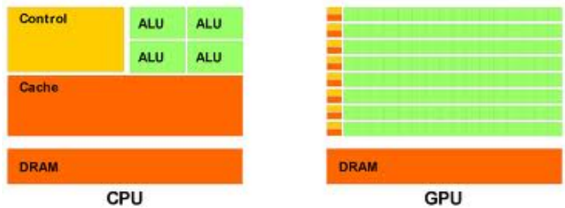
Figure 1.2: Architectural difference between a CPU (left) and a GPU (right). Green squares represent the arithmetic logic units (ALU) registers, yellow are the control registers and orange squares represent memory [15].
