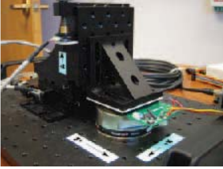
Fig. 5. The testing apparatus, including a three-axis linear stage, six-axis force transducer, and printed circuit board containing the three-axis tactile sensor.
