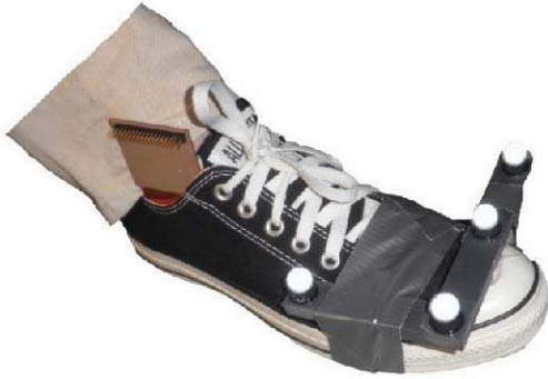
Fig. 5. Picture of insole in common shoe, with markers attached to examine angular deviations. Note the insole header passing out the lateral side of the ankle.
