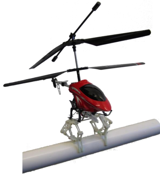
Fig. 1. Prototype mechanism attached to helicopter. Our mechanism, shown here attached to the skids on the bottom of an RC helicopter, uses a bilateral configuration of Sarrus-based linkages to passively grip cylindrical perches. The mechanical advantage converts the weight of the helicopter into an amplified force exerted onto the perch grip, which allows the system to resist disturbances.
