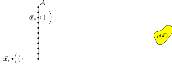
Figure 3.2. Physical setup for array imaging with an array \mathcal{A} of sources \vec{x}_s and a single receiver \vec{x}_r . The scatterer is represented by a compactly supported reflectivity function \rho(\vec{x}) .
