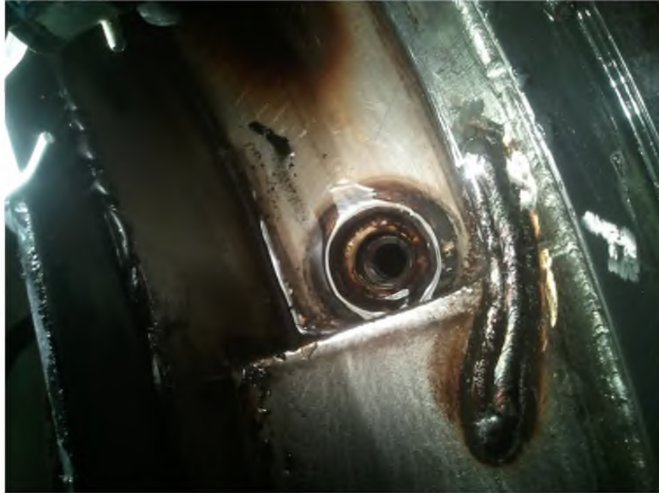
Figure 41 Repaired pedestal oil pan crack shown from above
