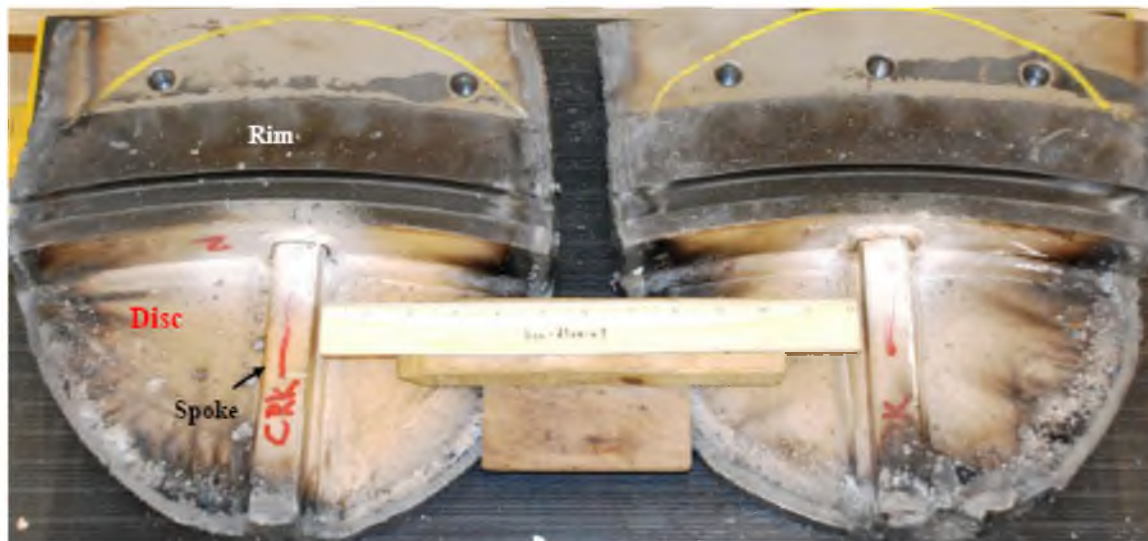
Figure 44 Bearing support sections containing cracks 1 & 2 at ends of the spokes
