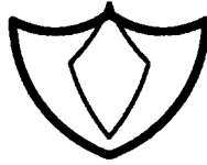
Figure 4.3: The outer lines surround the area of uncertainty with angles \alpha and \beta of 30^\circ and an error bound of \pm 10^\circ in each. The landmarks are at A, B and C. The inner area is for visual angles of 60^\circ with the same error bound. The landmarks are at A', B and C'.
