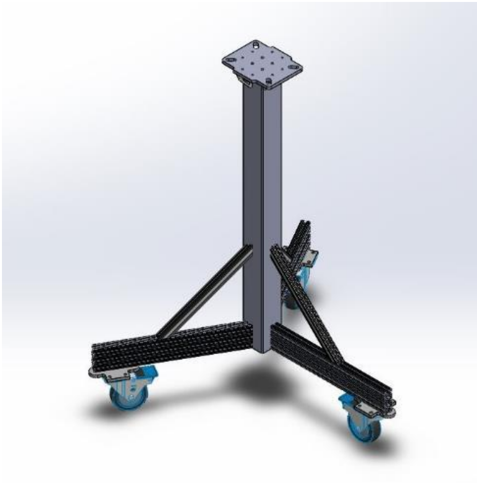
Figure 18. Drywall lift tripod base constructed from t-slot extrusion. Copyright 2016 by Mark Eilertsen
