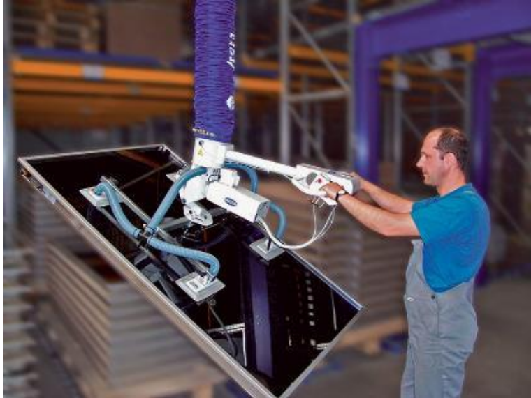
Figure 11. Example of a warehouse-based panel lift. Adapted from “Worker Lifting Solar Panels in Warehouse,” by Ergonomic Partners, n.d. Retrieved from https://www.ergonomicpartners.com/images/Jumbo-Ergo-Vacuum-lifter-lg.jpg Copyright 2016 Ergonomic Partners.
