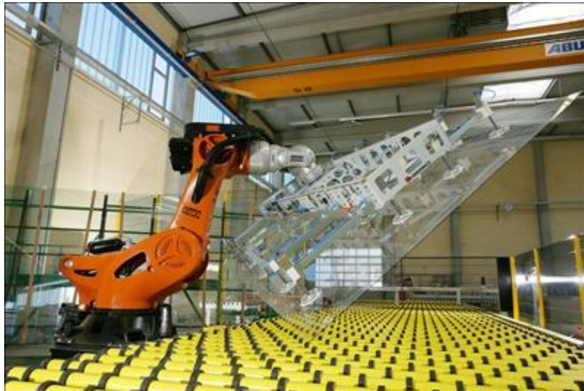
Figure 10. Industrial robot lifting panels. Adapted from “KUKA robot for flat glass handling,” by KUKA Roboter GmbH, n.d. Retrieved from https://en.wikipedia.org/wiki/KUKA#/media/File:KUKA_robot_for_flat_glas_handling.jpg . Copyright 2003 by KUKA Roboter GmbH.
