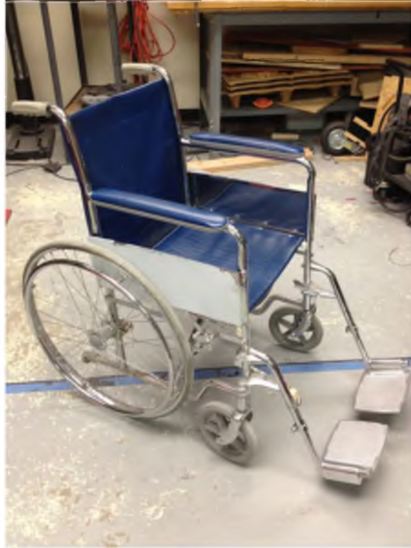
Figure 4 – Traditional wheel-rim propulsion wheelchair with sling seat and footrests.
