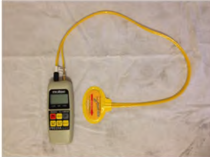
Figure 10 – Predia shear sensor, manufactured by Molten Corporation.
