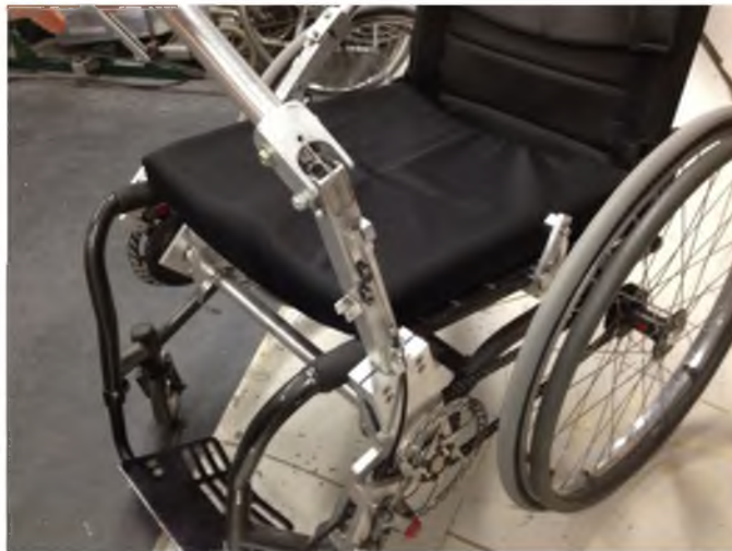
Figure 5 – Lever-arm wheelchair. Levers were attached with braking levers to actuate the chain and propel the wheel. The lever controls the corresponding wheel independently.
