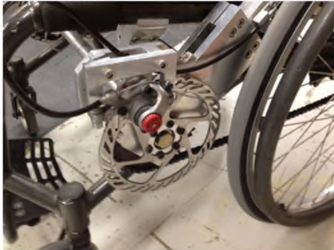
Figure 6 – Chain activation assembly. The calipers are compressed upon the rotor when the brake is applied from the hand lever. Upon application of brake, the lever is clamped to the rotor, rotating the wheel forward or backward.
