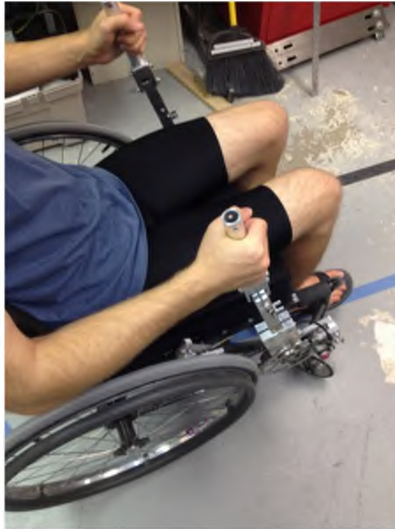
Figure 1 – Test subject wearing tight fitting short, experimenting with lever-arm wheelchair prior to testing.
