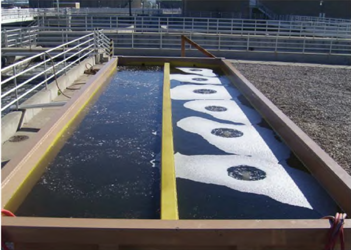
Figure 2- Overview of the pilot-scale reactor in operation. Control tank is on the left, Poo-Gloo tank is on the right.
