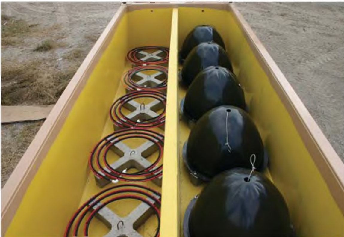
Figure 1- Overview of the pilot-scale reactor configuration. Control tank is on the left, Poo-Gloo tank is on the right (Nearest base and dome are out of the picture).
