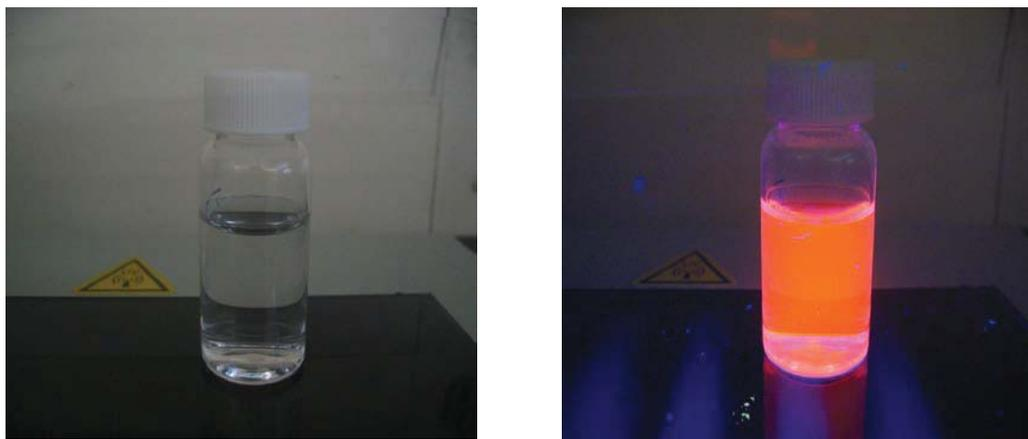
**Figure 3.2.** Red-emitting gold nanoparticle solutions on the UV transilluminator (excitation 254 nm)
