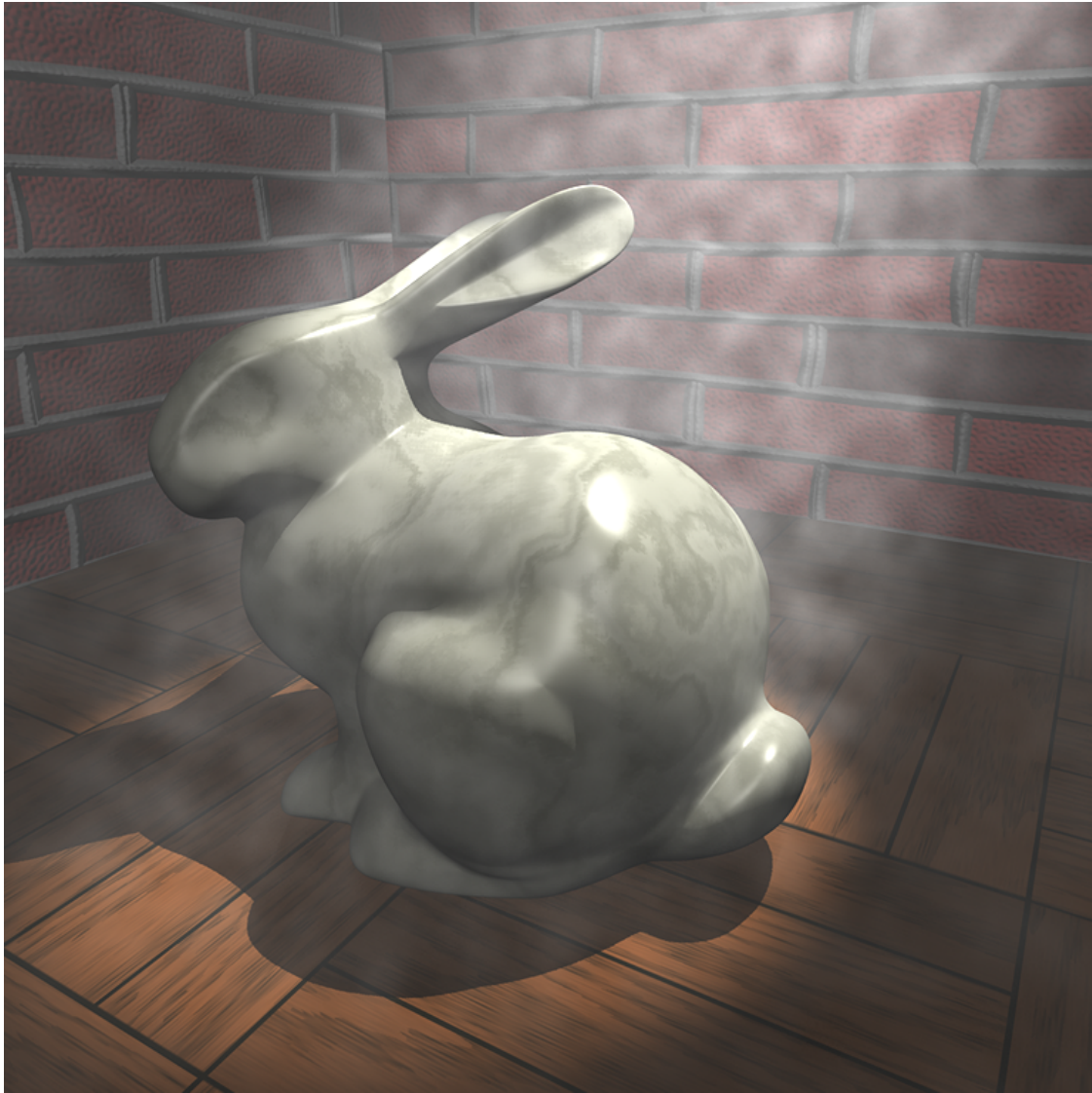
Figure 4.14. Rendered scene with fixed point version of our noise. Compare with Figure 4.1. All noise evaluations were performed with eight fractional bits and a 64-entry gradient table. While not identical, this shows that the modified algorithm with reduced precision can be a viable alternative to floating point Perlin noise.
