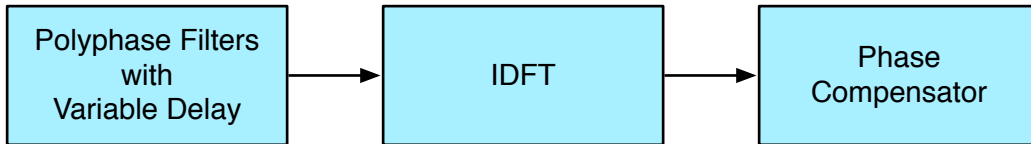
Figure C.1. Proposed architecture for adding a variable delay to the analysis filter bank. The phase compensator multiplies each subcarrier output by the appropriate amount.
