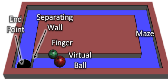
Figure 3.5. The virtual environment used for the ball manipulation experiment. For the experiment only the top view of the maze was visible and the virtual finger and ball were invisible. A wall between the start and end points prevented participants from moving the ball in the opposite direction. Image was taken with permission from Yazdian et al. [2013] © 2013 IEEE.
