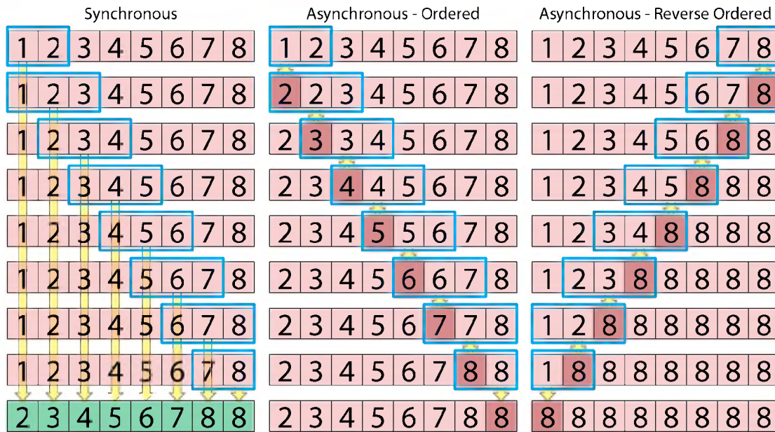
Figure 5.1. Comparison of synchronous and asynchronous updates of a 1D cellular automaton. The illustration shows only the first iteration in detailed steps. In the synchronous case, the original buffer is in red and the extra buffer for intermediate results is in green. Values are updated according to the maxima within the moving window (in blue), indicated by the yellow arrows. In the asynchronous cases, there is no extra buffer, so updates are immediate. The updated values in each step when the window moves are in dark red. We can repeat the iteration for the first two cases until all cells are updated to the maximum ID. Their results look exactly the same. The last case has already converged after the first iteration.
