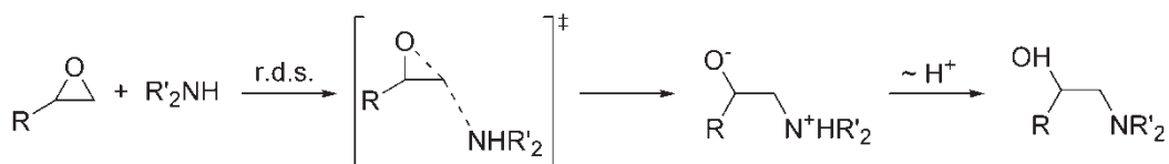
Scheme 2.1. The general mechanism of an epoxy-amine curing reaction. 8 (r.d.s. stands for rate determining step).
