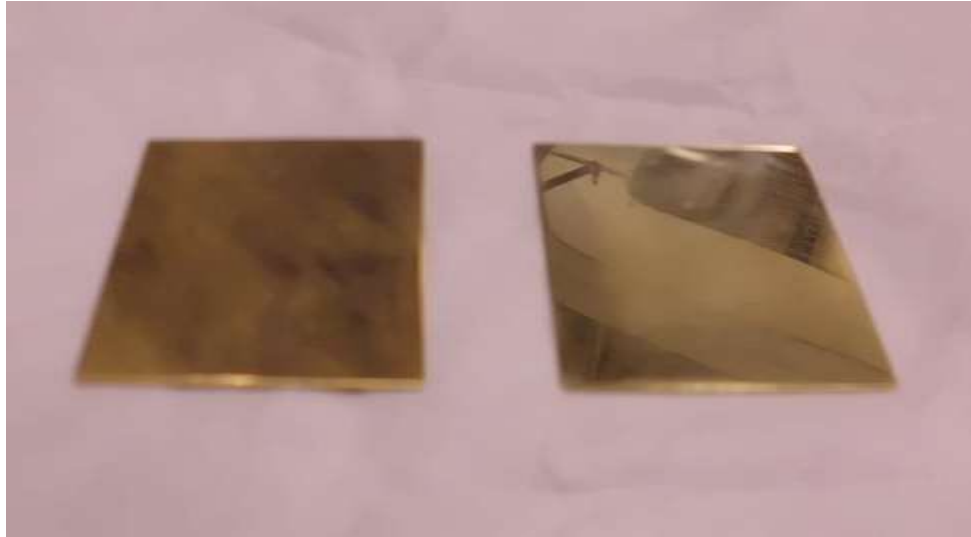
Fig. 3.8 Comparison of unpolished and polished brass partition pieces.
