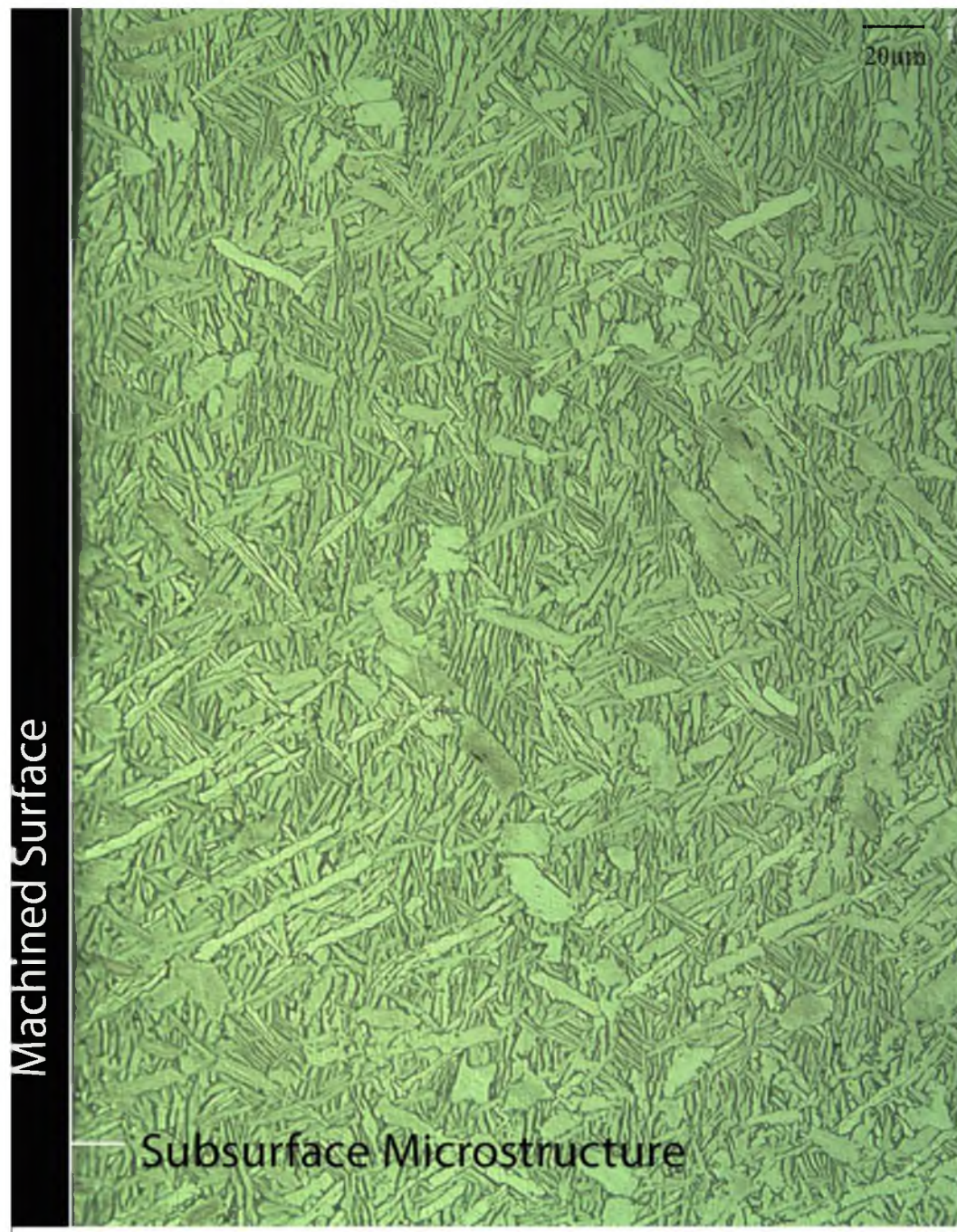
Figure 4.6: Ti-6Al-4V subsurface microstructure developed when machined using flat-faced uncoated cutting tool insert and dry machining condition.
