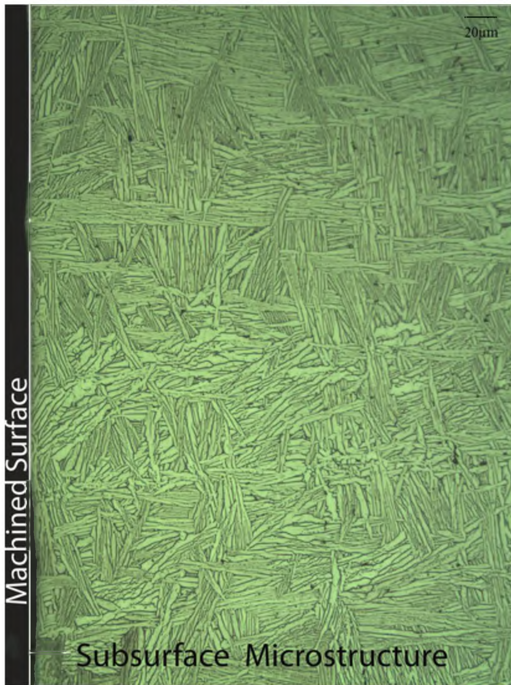
Figure 4.8: Ti-6Al-4V alloy subsurface microstructure developed when machined using grooved multilayered CVD coated cutting tool insert and dry machining condition.
