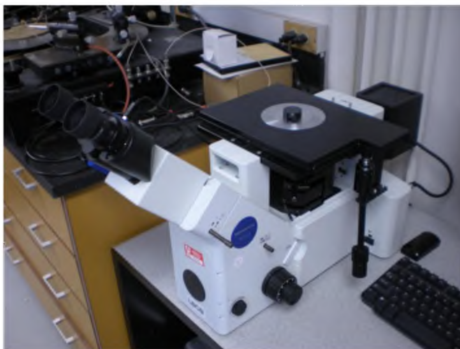
Figure 3.10: Epoxy mould mounted at the base of the optical microscope.
