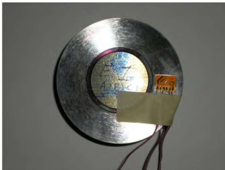
Figure 3.2: Machined Ti6Al4V alloy work-piece, ready for residual stress measurement.
