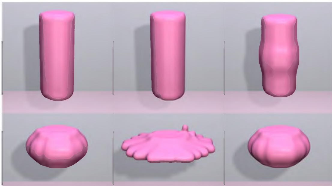
Figure 4.8. Final frames in a comparison of our method (left) against a method that uses a rest configuration (middle) and a method with an additive strain model (right). The top row is an elastic material, the bottom row is a very plastic material. The simulation consists of applying and then releasing an analytic compression force that increases away from the center of the object. The lower middle image is the last frame before the simulation became unstable.
