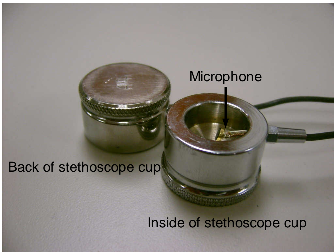
Figure 4.1 Metal stethoscope cup used to attenuate ambient sounds and amplify tracheal sounds.
