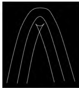
Figure 6.2: Uniform offsets may introduce crossings.
