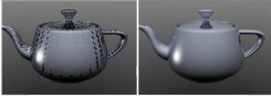
Figure 3.5: Left: Failure to adjust tolerances may result in surface acne. Right: Properly adjusted tolerances solve the problem. Black regions result from truncated ray depth.
