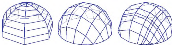
Figure 7.3: Angular parameters on the hemisphere. The standard \theta, \phi spherical parameterization results in poor knot spacing (left). Our trimmed square-to-sphere mapping is much more uniform (middle). Nonuniform knot spacing can be used with our mapping, to better approximate a highlight for example (right).
