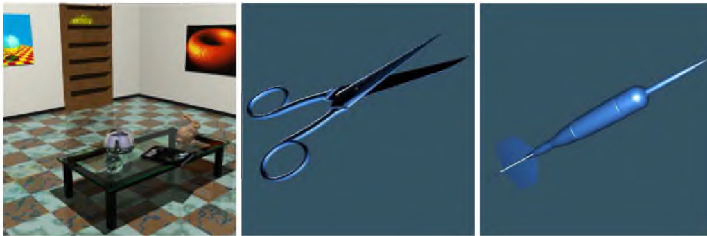
Figure 3.14: Ray traced Bézier surfaces from the interactive ray tracing paper by Parker et al. [1]. Reprinted with permission. © Copyright 1999 by ACM, Inc. Definitive version: http://doi.acm.org/10.1145/300523.300537 .
