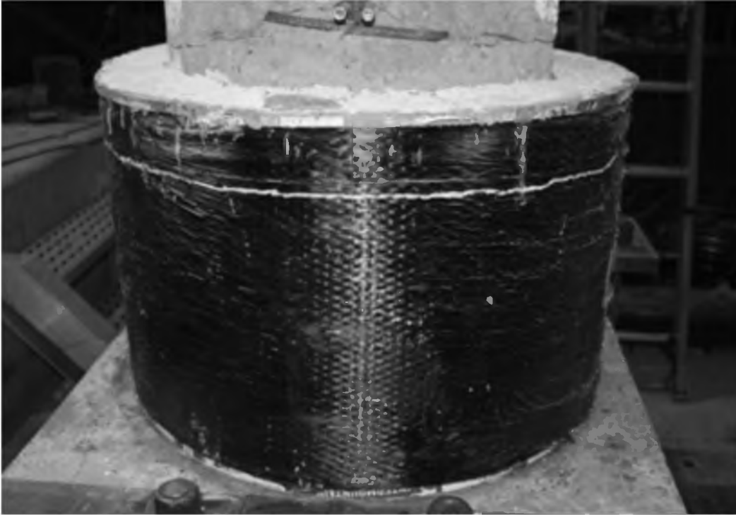
Figure 4.6 – Transverse CFRP crack located just above white line
