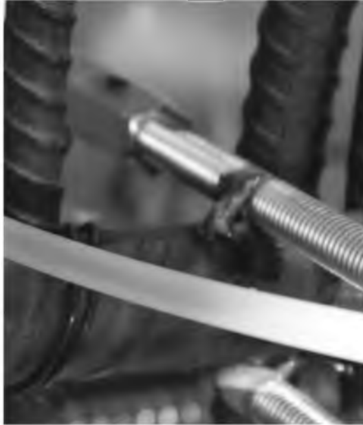
Figure 4.15 – Typical tack weld used to connect LVDT rods to the column longitudinal rebar
