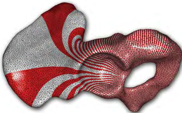
Figure 1.3. Sweeping can cause significant of parametric distortion, if the object is irregular.
