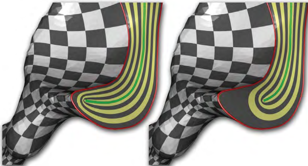
Figure 5.9. A trim value m_0 closer to 1 (right) can introduce parametric distortion, but favors the periodic parameterization. A smaller trim values favors the polycube parameterization.
