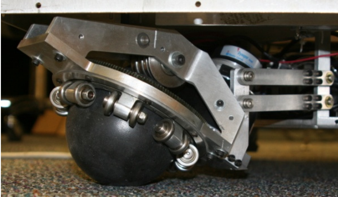
Figure 1.4: Omnidirectional Ball Wheel mechanism on the wheelchair used for this research.
