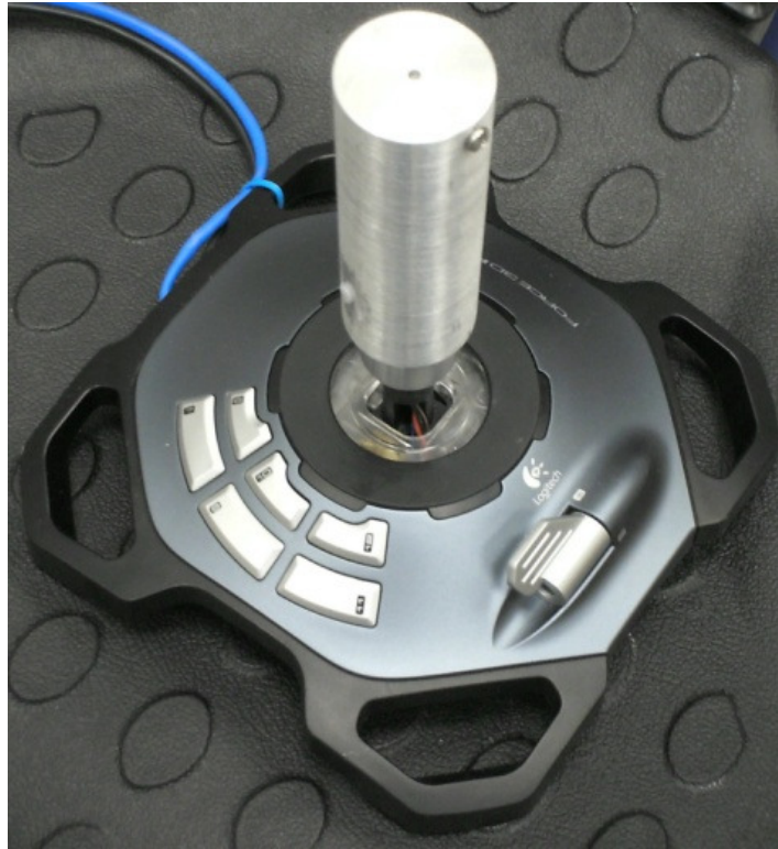
Figure 2.2: Modified Logitech Force Pro gaming joystick. Rotational feedback is provided by a Maxon gear head motor enclosed in the handle. Handle provides about 180° of rotation.
