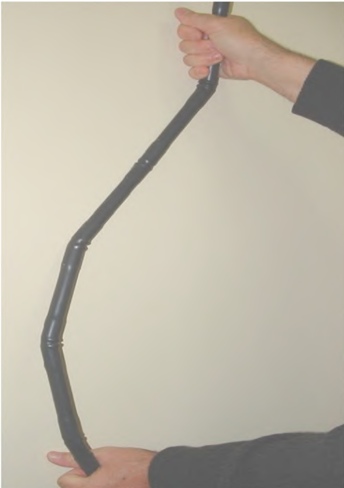
Figure 2-6. Rigid segments connected at joints allowing the SAA to move freely and monitor lateral deformation (courtesy of Measurand Inc. www.measurand.com ).
