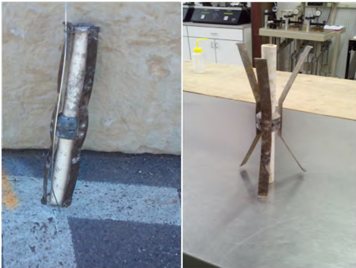
Figure 2-3. A spider magnet is shown in two positions: The legs of the spider magnet are closed (left), and the legs of the spider magnet are extended (right).
