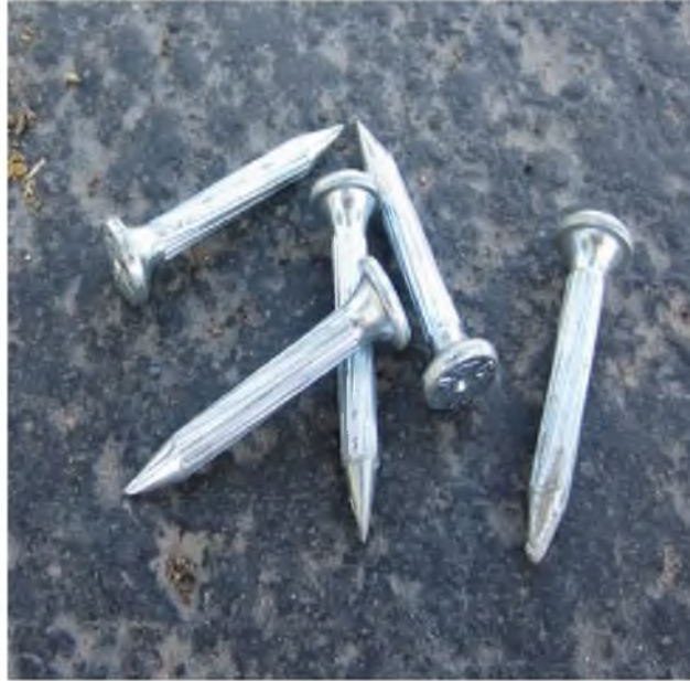
Figure 2-10. Parker Kalon (PK) nails used for measuring postconstruction settlement at the bridge approach.
