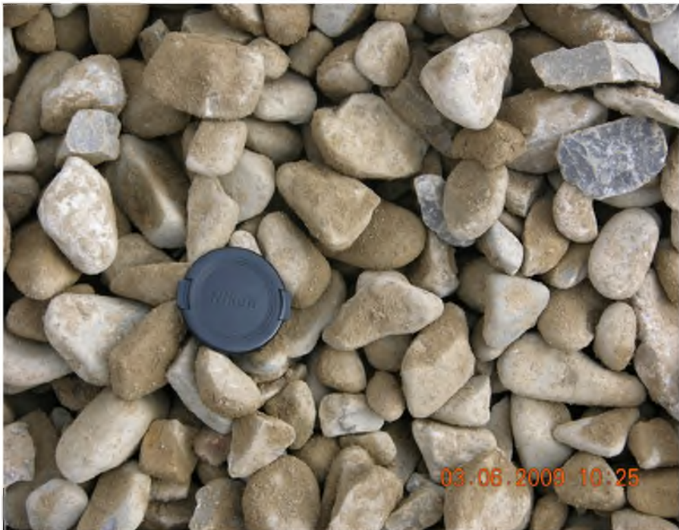
Figure 1-8. Closeup of borrow material. Camera lens cap shown for scale.
