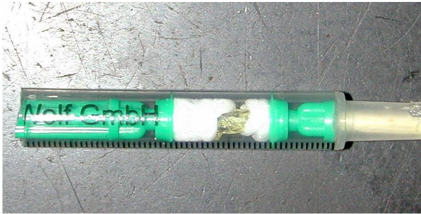
Figure 3.6 – Mineral particles are confined by Styrofoam layers in a syringe tube.
