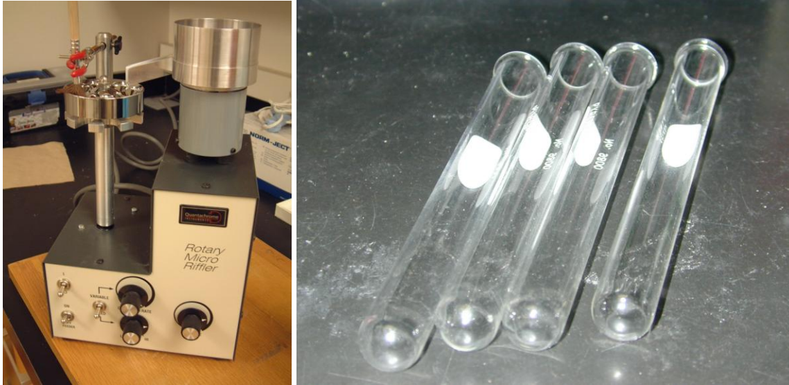
Figure 3.4 – Rotary Micro Riffler and testing tubes.
