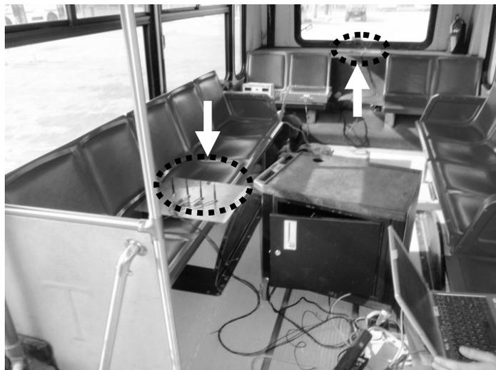
**Figure 5.2: Photo of rear half of bus with measurement equipment at location 24 for TX2, marked by large white arrows (see also Figure 5.4).**
