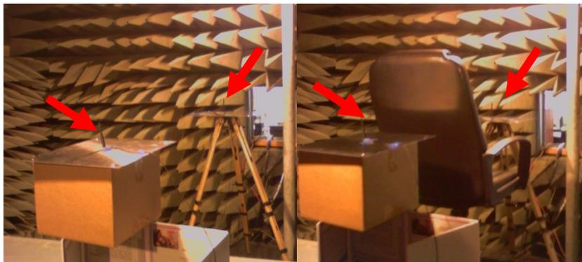
**Figure 3.18: Photo of SISO equipment setup with and without chair, with red arrows pointing to transmit and receive antennas.**
