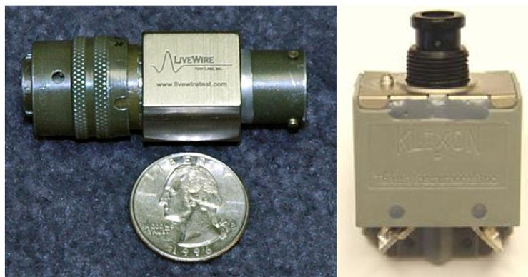
**Figure 1.1: Smart Connectors (Left) and Arc Fault Circuit Breakers (right, approx. 1” square) are two applications currently being commercialized. Current data links are infrared or hard-wired. Wireless communication will enable large-scale deployment in regions of the aircraft that are otherwise inaccessible.**
