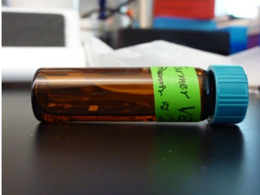
Figure 29 Test setup for 5-day VEGF diffusion test. A PDMS device filled with 14.5uL 10ug/mL VEGF was placed in the glass amber vial with 1mL PBS as the receiver chamber medium
