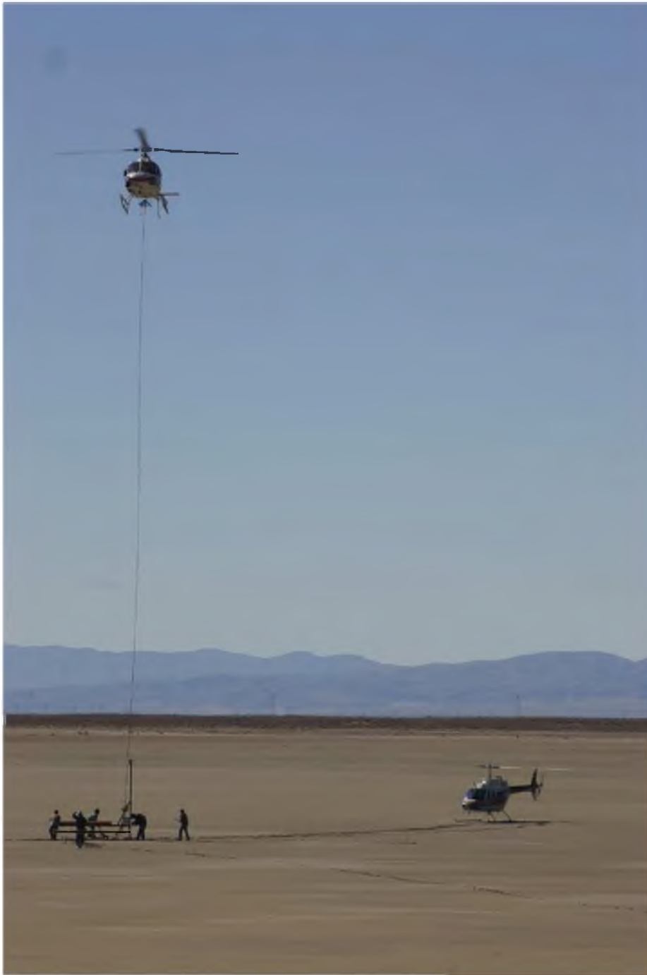
Figure 3.7. Image of field deployment of a Surface Detector (SD) via helicopter: one helicopter brought the SD itself, while a second helicopter ferried a crew from site to site to receive the SD, align it, and turn it on.
