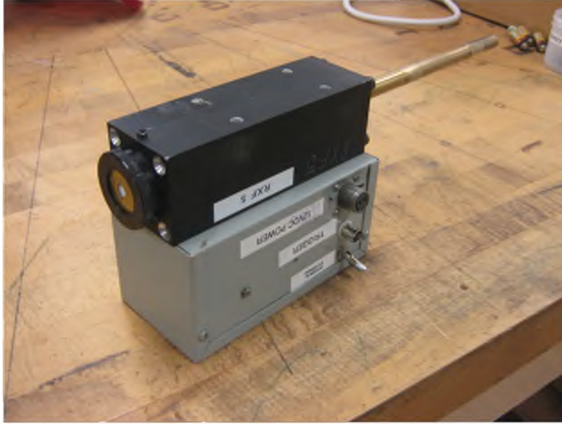
Figure 3.19. This is a photograph of the close up view of the Roving Xenon Flasher (RXF). Shown is the long post for mounting the RXF on each mirror, the black box which contains the flash lamp, and the grey box containing the power source.
