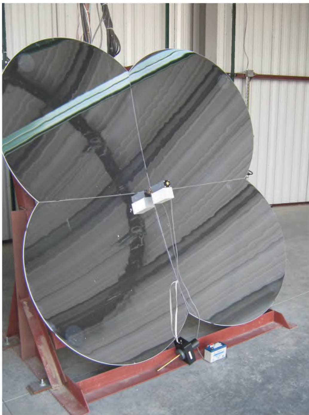
Figure 3.20. A photograph of the Roving Xenon Flasher (RXF) positioned at the center of the mirror where it illuminates the PMTs in the camera: the UVLED has been removed from its position at the center of the mirror to make space for the RXF.
