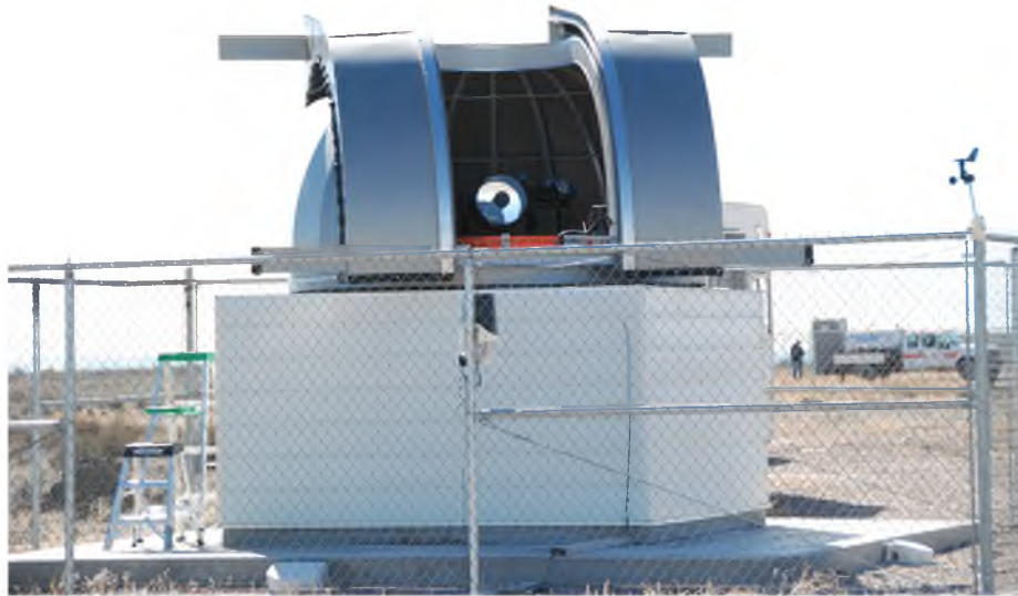
Figure 3.27. This photograph shows the monostatic LIDAR facility located at the Black Rock Mesa Fluorescence Detector (BRMFD). It houses a Nd: YAG laser used for measuring the Vertical Aerosol Optical Depth (VAOD).
