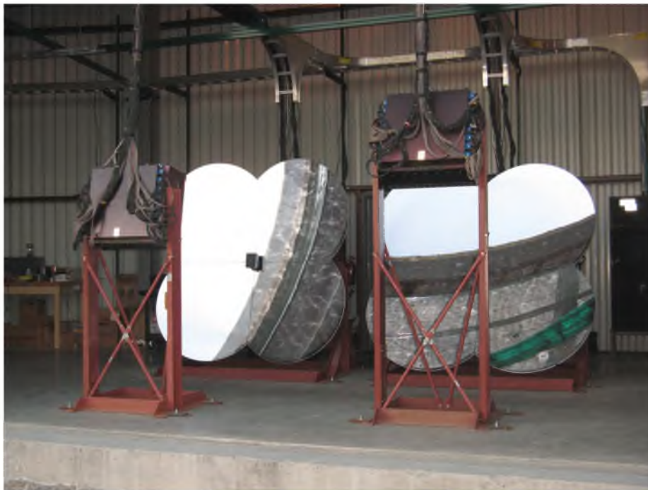
Figure 3.15. A pair of telescopes at the Middle Drum Fluorescence Detector (MDFD): in the photo, the telescope on the right views 3^{\circ} - 17^{\circ} above the horizon, while the one on the left views 17^{\circ} - 31^{\circ} above the horizon. Thus, the pair view 28^{\circ} in elevation and the seven pairs of telescopes view 112^{\circ} in azimuth.
