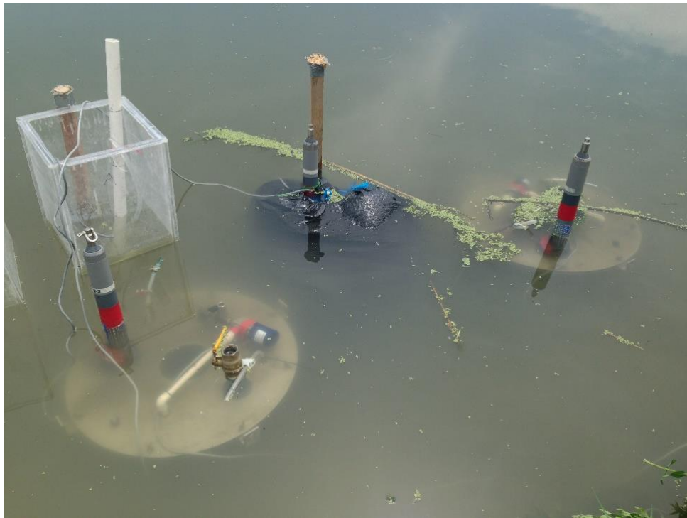
Figure 3.3, SOD Chambers Deployed at Site
