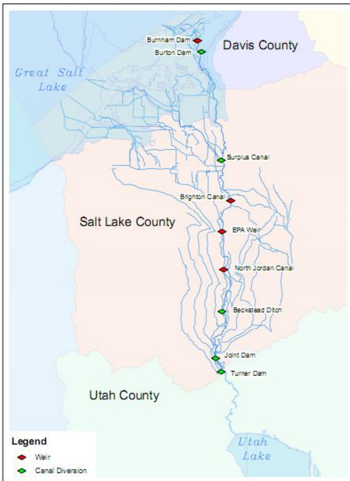
Figure 2.2, Major Diversions, Canals, and Flow Control Structures (Hogsett, 2015)
