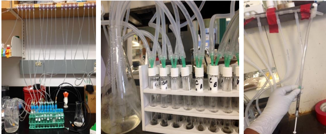
Figure 3.6, Experimental Setup for Denitrification Rate Using ^{15}\text{NO}_3^- Substrates
