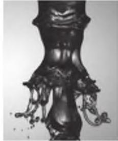
**Figure 2.9.** Fiber-type breakup morphology © [41].
