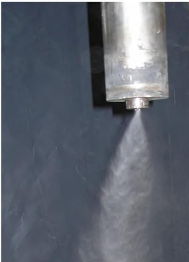
**Figure 3.5.** Old atomizer design showing a nonconcentric spray.
