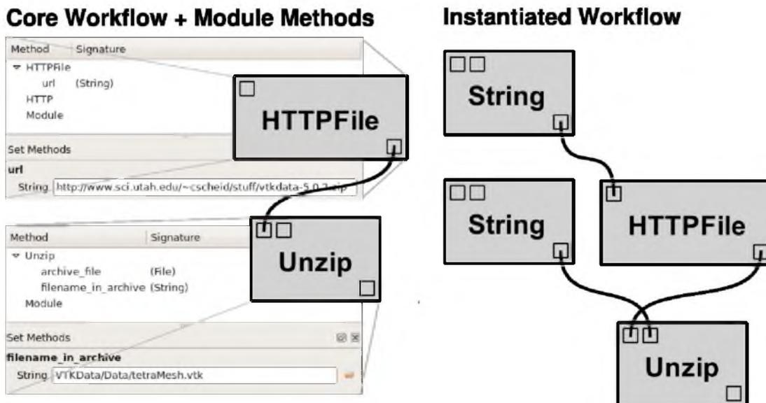
**Figure 6.7:** When a workflow is scheduled for execution, the methods of a module are instantiated as additional executable modules. This simplifies the implementation of `Module` subclasses by VisTrails users, and the interplay of method specification and caching functionality.
