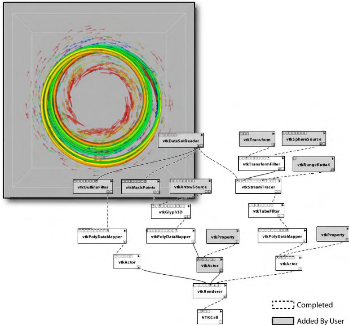
**Figure 5.6:** One of the test visualization pipelines applied to a time step of the Tokamak Reactor dataset. VisComplete could have made many completions that would have reduced the amount of time creating the pipeline. In this case, about half of the modules and completions could have been completed automatically.
