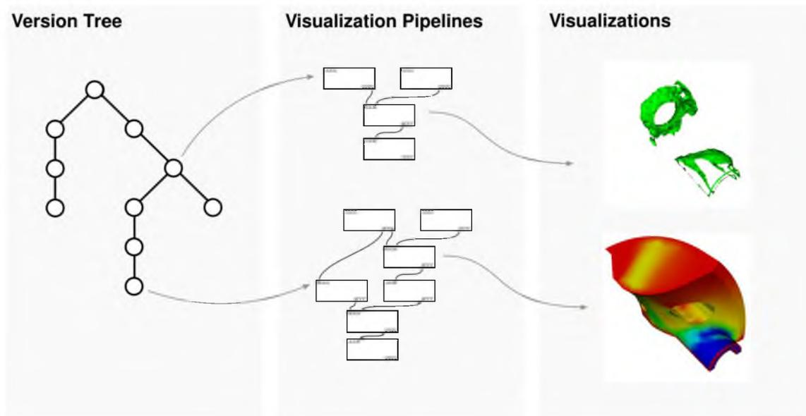
**Figure 3.1:** A review of terminology from VisTrails. The *version tree* (shown on the left) captures the history of the exploration process, where each node corresponds to a *visualization pipeline*. Edges in this tree are functions from  $f : \mathbb{V} \rightarrow \mathbb{V}$ . Each pipeline comprises *modules*, *connections*, and *parameter values*, and generates a *visualization* (shown on the right).
