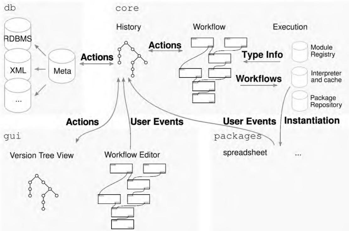
**Figure 9.1:** A high-level view of the `VisTrails` architecture. The main application is comprised of three high-level, mostly independent components: `VisTrails` core, `VisTrails` db, and `VisTrails` gui. The arrows indicate the major interactions between the subsystems.
