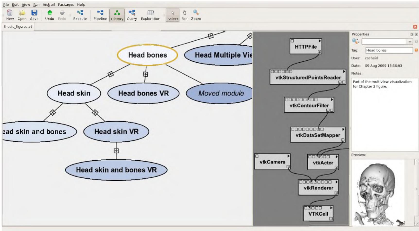
**Figure 3.2:** An overview of the main VisTrails GUI. Shown on the left side is the version tree view, where users can navigate the captured history of the exploration process. In the middle, we show the highlighted workflow, and associated notes and thumbnail on the right side.
