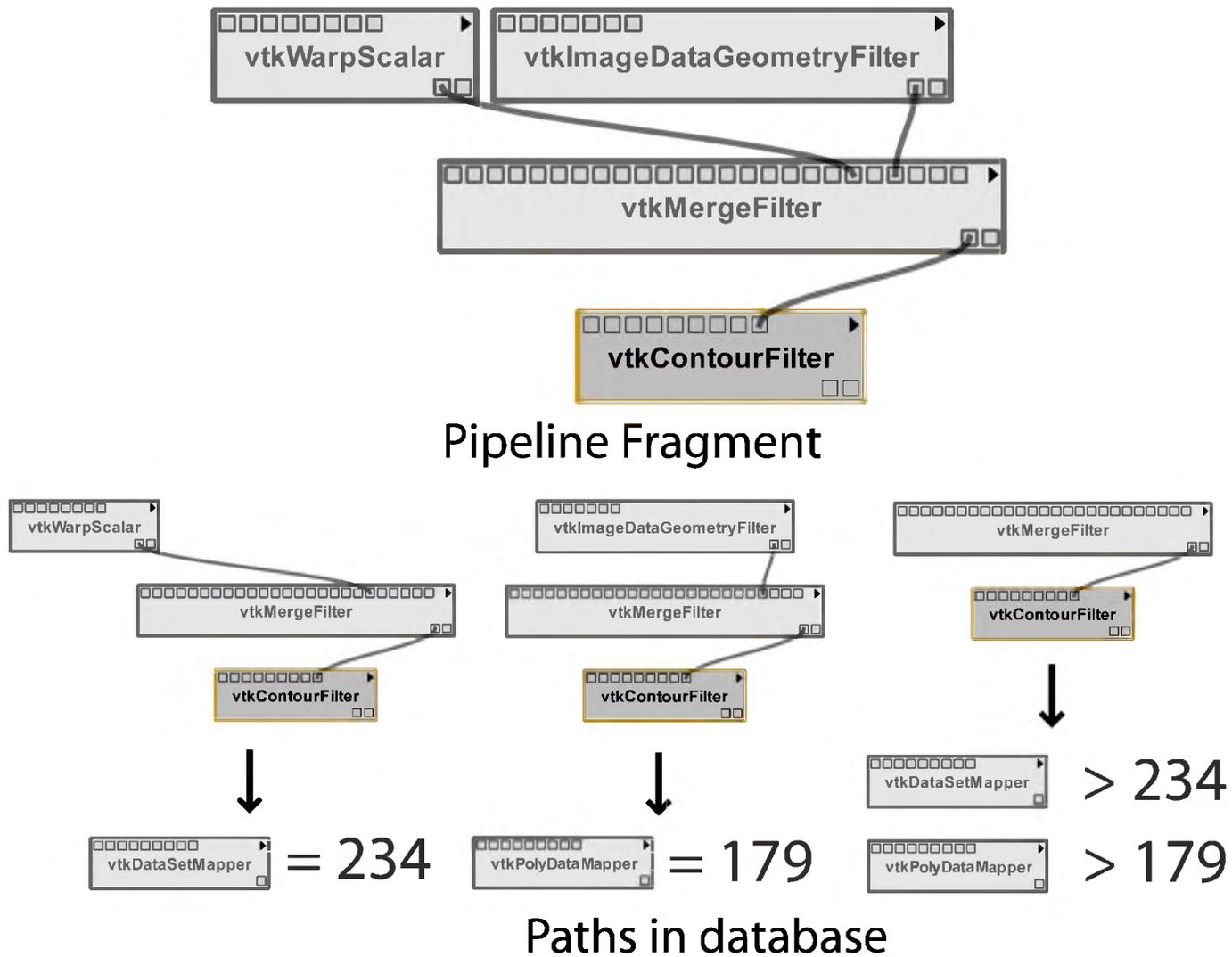
**Figure 5.5:** At each iteration, we examine all upstream paths to suggest a new downstream vertex. We select the vertex that has the largest frequency given all upstream paths. In this example, “vtkDataSetMapper” would be the selected addition.
