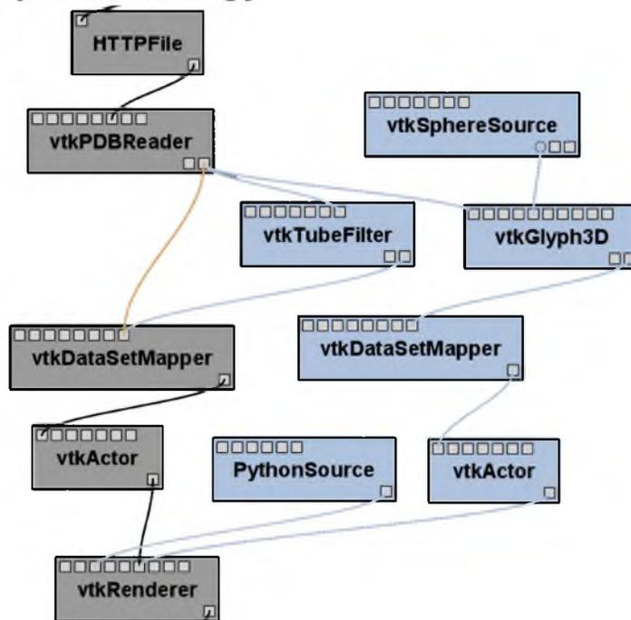
**Figure 4.2:** Example of an analogy between pipelines where there is no perfect module matching. The difference in the left pipeline pair is transferred to the right pipeline pair. Note, however, that the modules are not the same—the system must find the most likely pairing based on the similarity measure described in the text.
