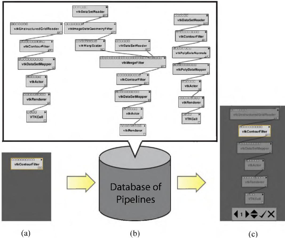
**Figure 5.1:** The VisComplete suggestion system and interface. (a) A user starts by adding a module to the pipeline. (b) The most likely completions are generated using indexed paths computed from a database of pipelines. (c) A suggested completion is presented to the user as semitransparent modules and connections. The user can browse through suggestions using the interface and choose to accept or reject the completion.
