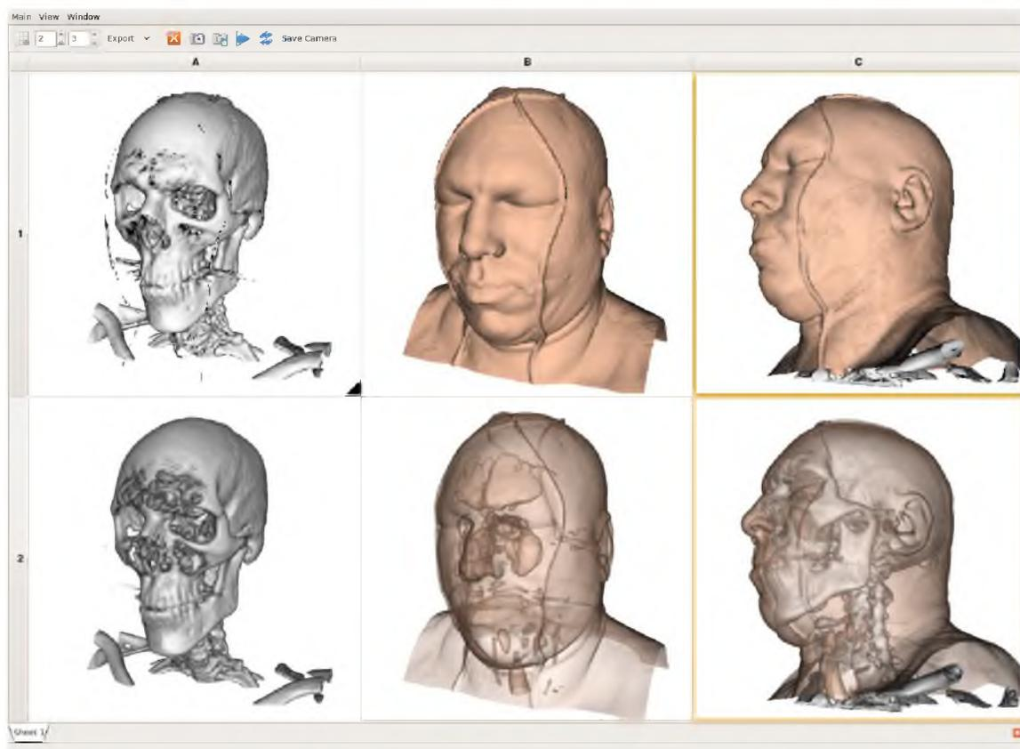
**Figure 2.1:** VisTrails provides support for multiple-view visualization via the VisTrails Spreadsheet. Cameras as well as other vistrail parameters for different cells can be synchronized. This spreadsheet shows visualizations of the Visible Human dataset using different algorithms. The top row shows the rendering of two isovalues, while in the second row, images are created using volume rendering. The cameras for the cells in the rightmost column in the spreadsheet above are synchronized.
