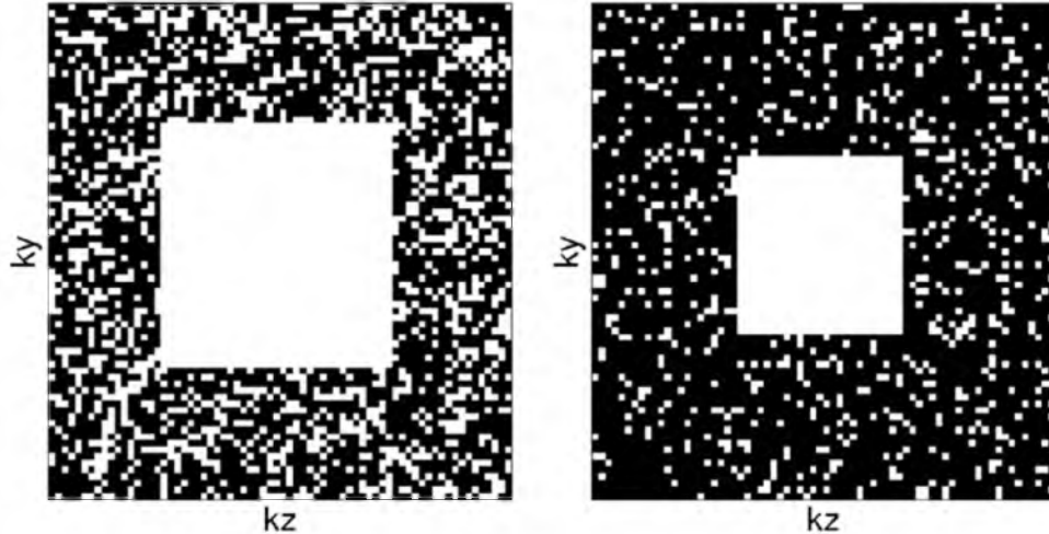
Figure 3.2: Two-dimensional representation of sampling masks in the phase-slice plane for 50% (left) and 75% (right) undersampling. The data were sampled fully in the readout direction.
