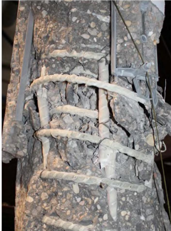
Figure 2.18: Failure details of column #4T-DB1
