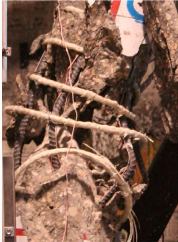
Figure 2.19: Failure details of column #5T-SS1
