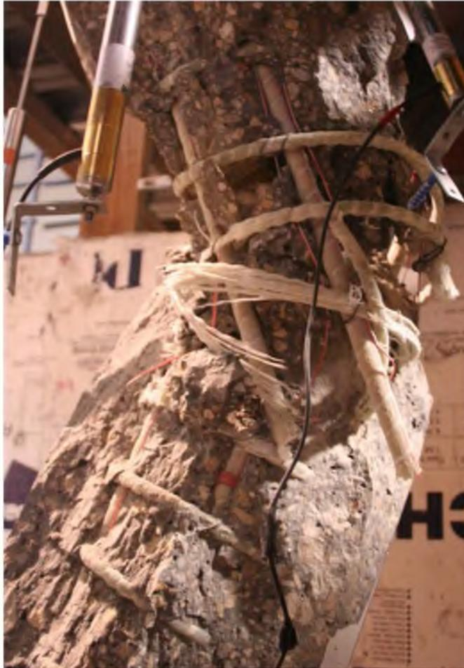
Figure 2.20: Failure details of column #6T-SG1
