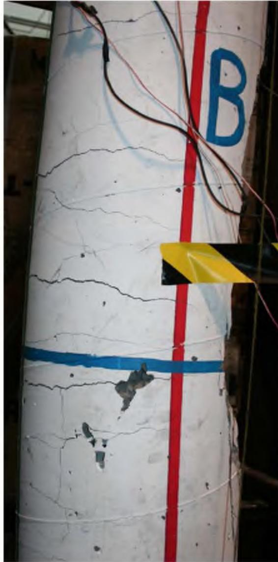
Figure 2.31: Failure details of column #7T-DB4
