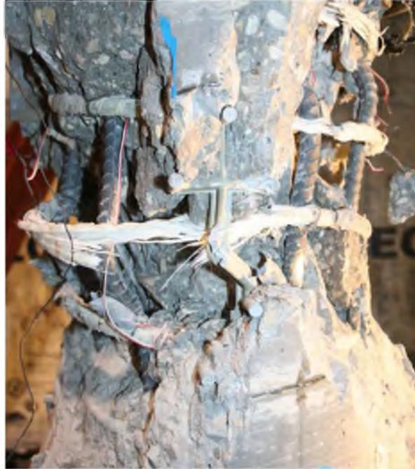
Figure 2.10: Failure details of column #2S-SS0
