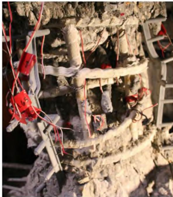
Figure 2.9: Failure details of column #1S-DB0
