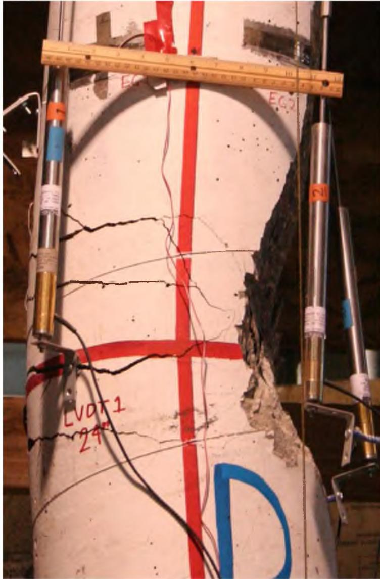
Figure 2.32: Failure details of column #8T-SS4
