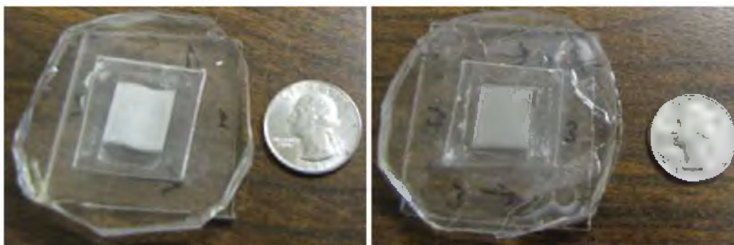
Figure 8.2: The pictures of two assembled MRI phantoms (left: with curved channels, right: with straight channels) along with a US quarter coin. Each phantom is placed in a square water reservoir formed by the PDMS cap and PDMS substrate. No air bubble can be seen in the phantom assembly.
