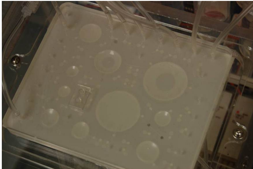
Figure 1: PDMS lab-on-a-chip used for DNA extraction.
