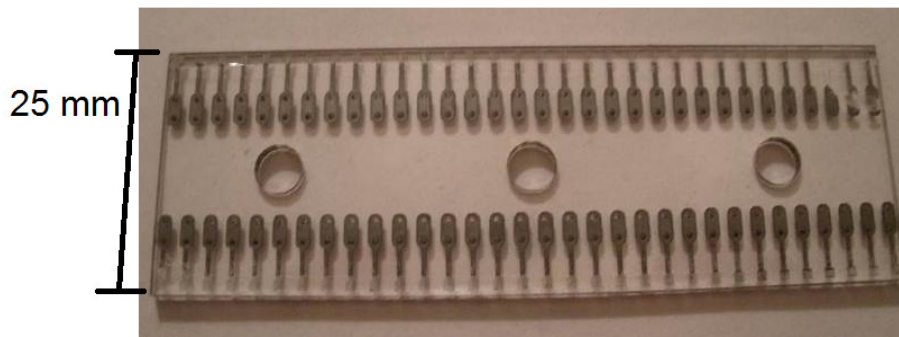
Figure 19: Array of 64 valves on a single PMMA chip. This chip is the size of a standard microscope slide.
