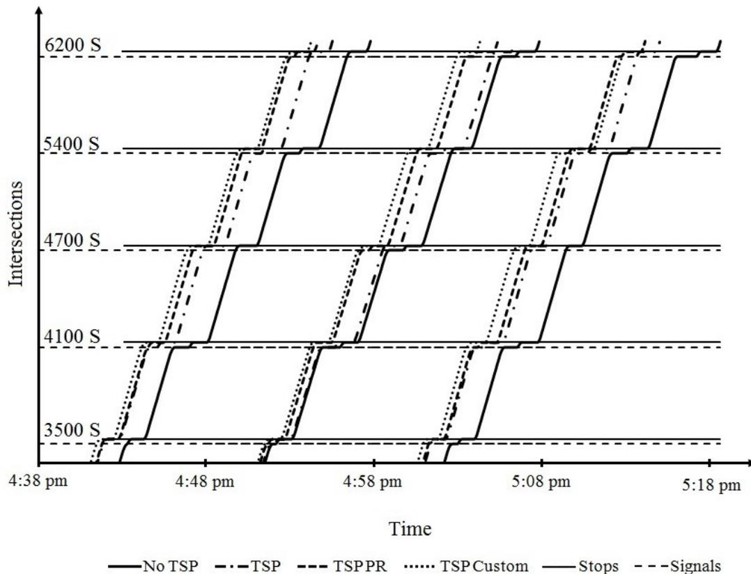
**FIGURE 7.3 BRT time-space diagram: three SB BRT vehicles.**
