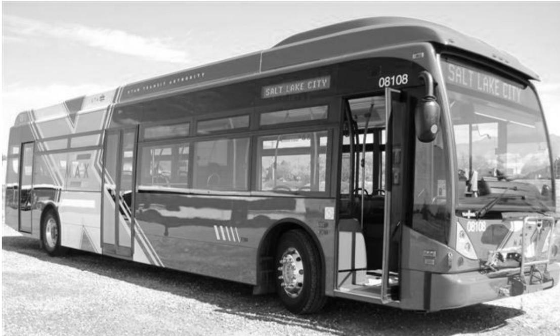
**FIGURE 4.5 Customized Van Hool A300 bus assigned to 35M line.**
