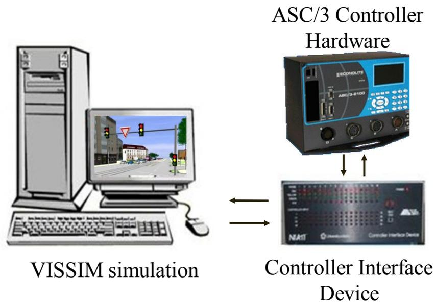
**FIGURE 6.1 ASC/3 – VISSIM HIL concept.**
