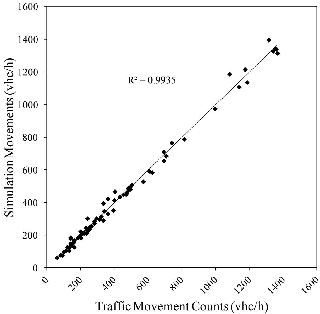
**FIGURE 7.2 VISSIM model calibration.**
