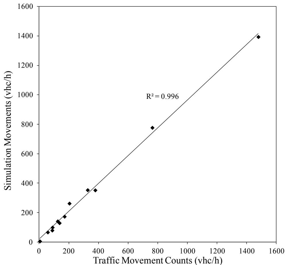
**FIGURE 8.3 VISSIM model calibration.**
