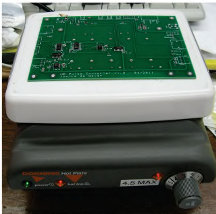
Figure A.5: A hot plate was used to solder surface mount components.
