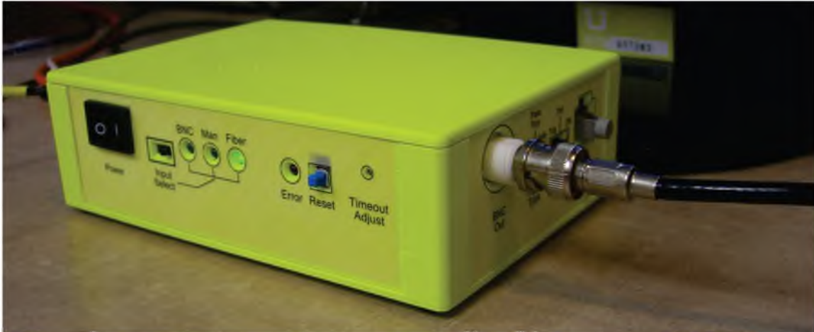
Figure A.1: Final version of the trigger conversion device. Front panel has an input select switch and LED indicators that display which input method is active, an error LED that illuminates when the safety timer has expired, a manual reset button to reset the device, and a safety timer adjustment screw. The output signals are on the right hand side of the device. Both electrical and optical outputs are active simultaneously. Between the outputs are two switches that select the trigger type and output mode.
