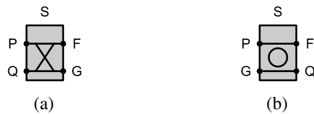
Fig. 3.14 Ports of two functionally equivalent optical logic building blocks: (a) Directional coupler-based logic gate (b) Ring-based logic gate
