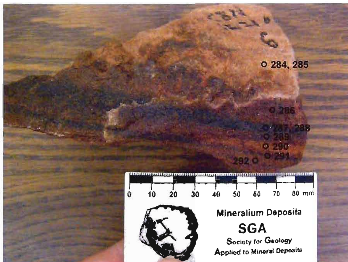
Figure A.19. Reflectance spectra transect across sample CBN 12.21.06#6. Numbers correspond to individual spectral analyses.
