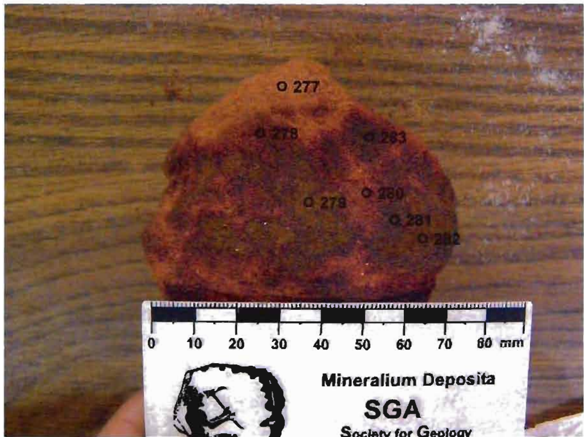
Figure A.18. Reflectance spectra transect across sample CBN 12.21.06#2. Numbers correspond to individual spectral analyses.
