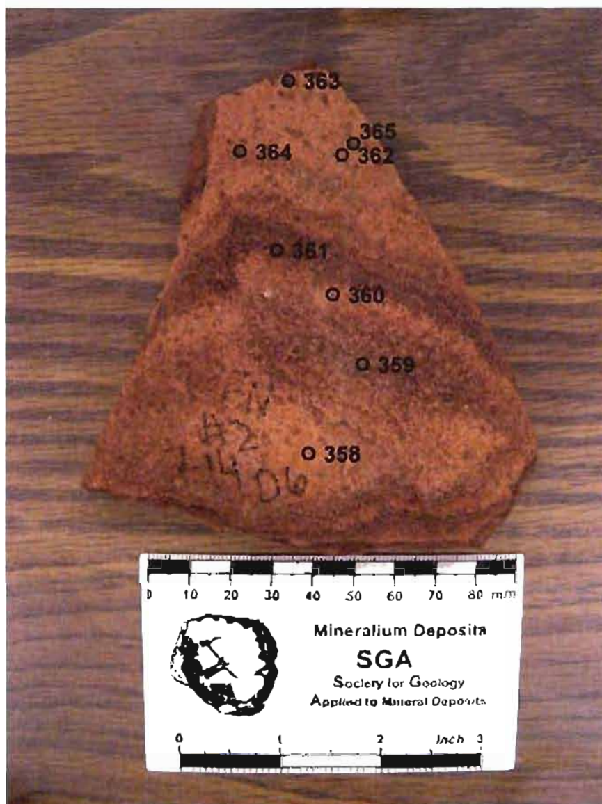
Figure A.27. Reflectance spectra transect across sample CBN 7.14.06#2. Numbers correspond to individual spectral analyses.
