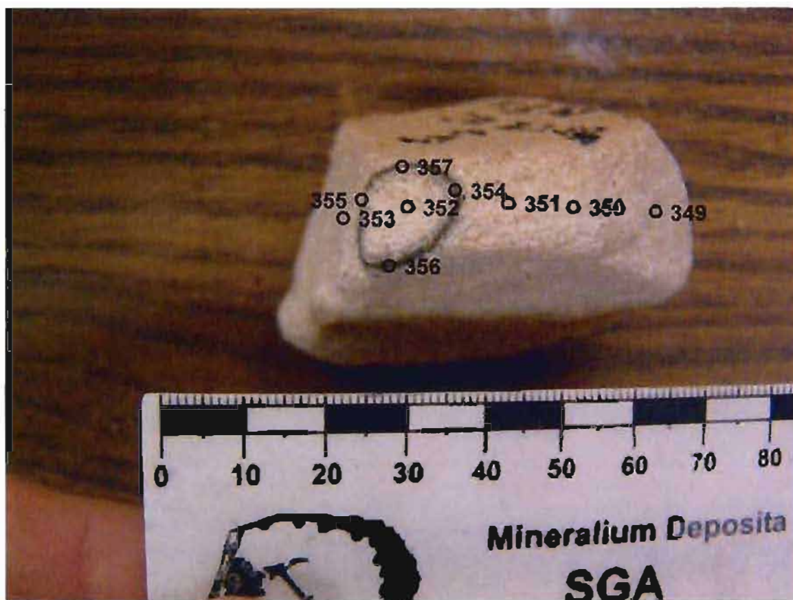
Figure A.26. Reflectance spectra transect across sample CBN 12.21.06#5. Numbers correspond to individual spectral analyses.
