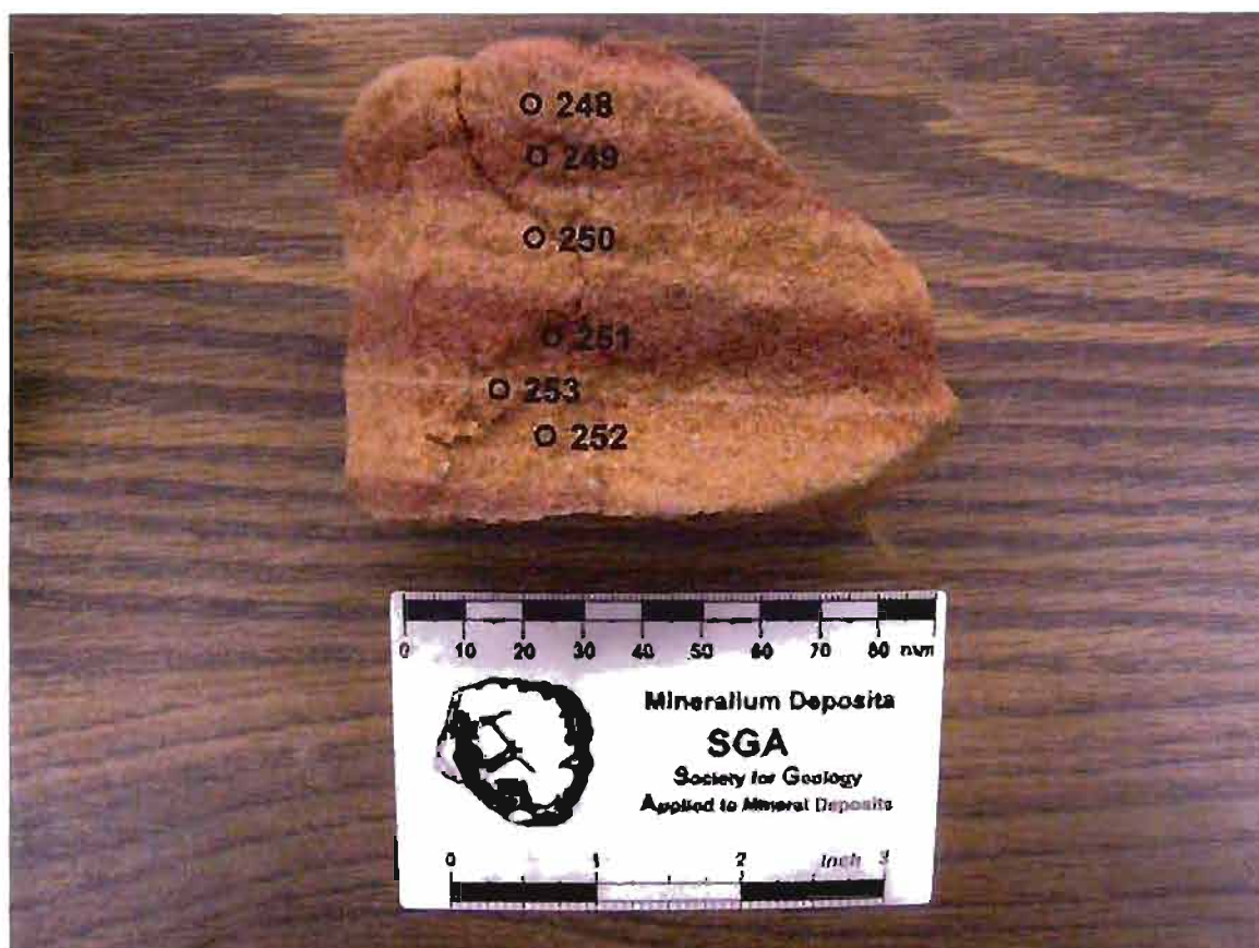
Figure A.15. Reflectance spectra transect across sample CBN 12.20.06#5. Numbers correspond to individual spectral analyses.
