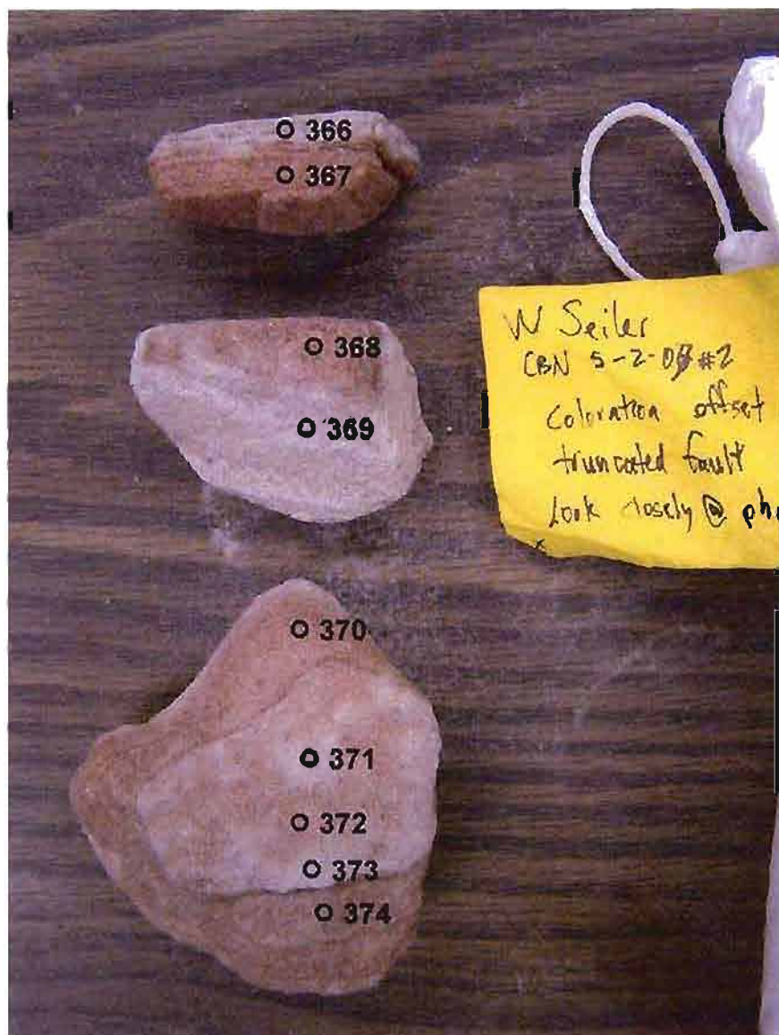
Figure A.28. Reflectance spectra transect across sample CBN 5.2.07#2. Numbers correspond to individual spectral analyses.
