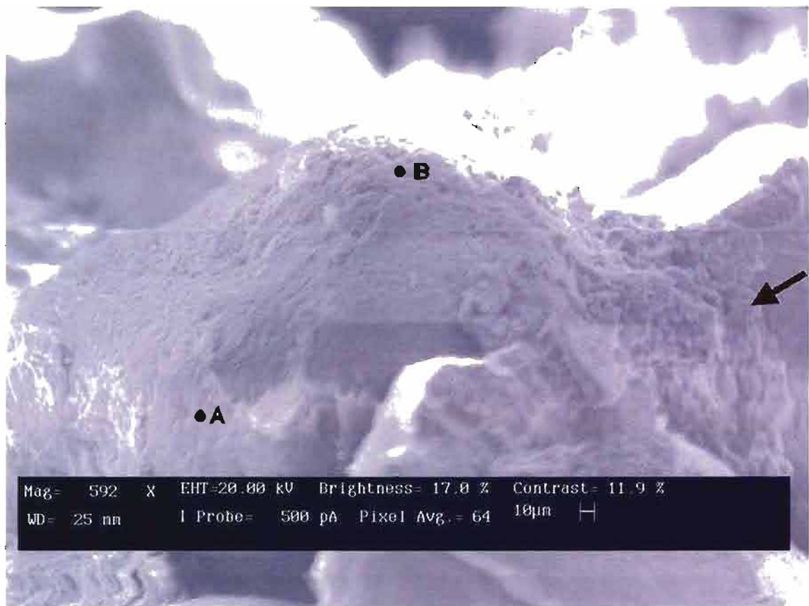
Figure A.7. SEM image of variable Liesegang atop red and white banded sample CBN 12.21.06#6. Letter A and B corresponds to EDAX analyses reported in Tables A.17 and A.18. Textured iron oxide grain coating imaged throughout, best viewed at right (arrow).
