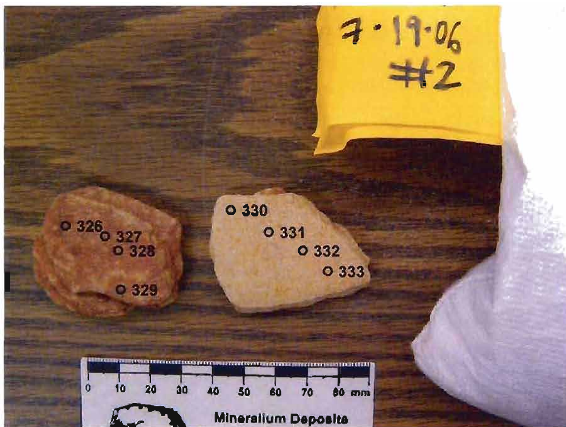
Figure A.23. Reflectance spectra transect across sample CBN 7.19.06#2. Numbers correspond to individual spectral analyses.
