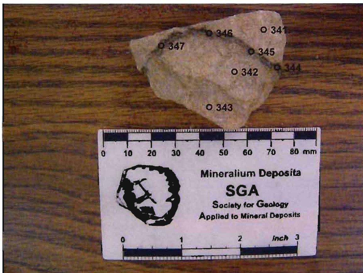
Figure A.25. Reflectance spectra transect across sample CBN 7.20.06#4. Numbers correspond to individual spectral analyses.
