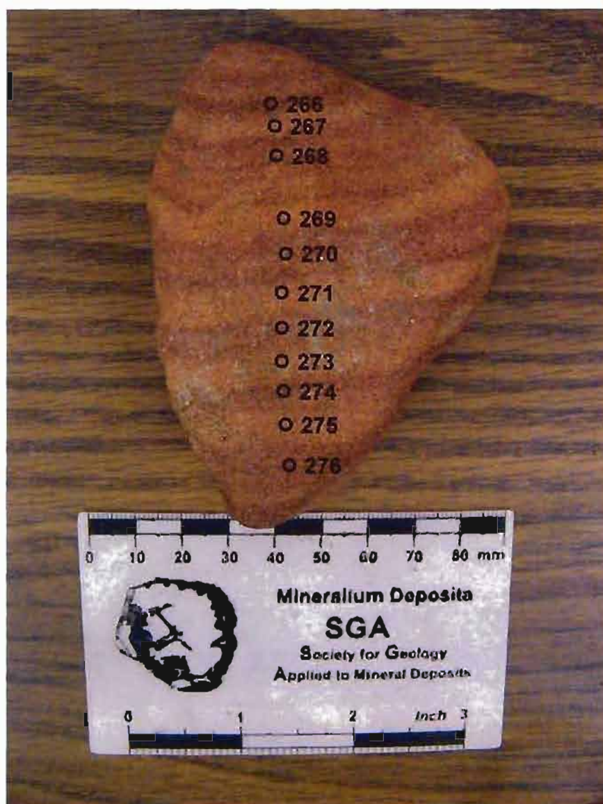
Figure A.17. Reflectance spectra transect across sample CBN 12.20.06#4. Numbers correspond to individual spectral analyses.
