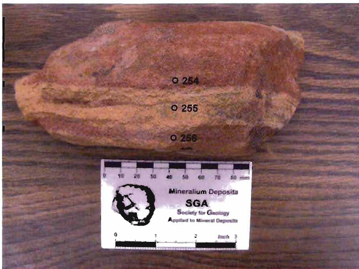
Figure A.16. Reflectance spectra transect across sample CBN 12.20.06#5. Numbers correspond to individual spectral analyses.
