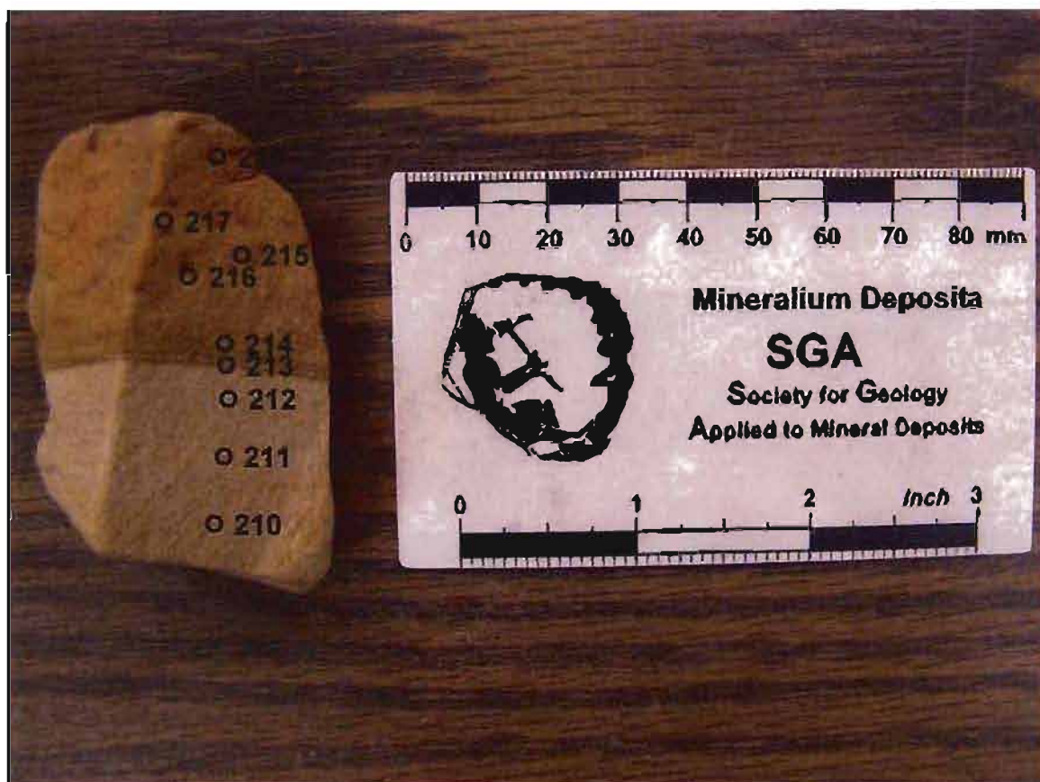
Figure A.12. Reflectance spectra transect across sample CBN 7.22.06#2. Numbers correspond to individual spectral analyses.
