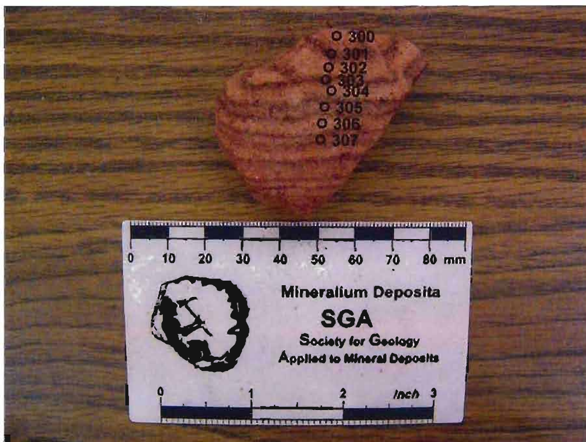
Figure A.21. Reflectance spectra transect across sample CBN 7.15.06#9. Numbers correspond to individual spectral analyses.
