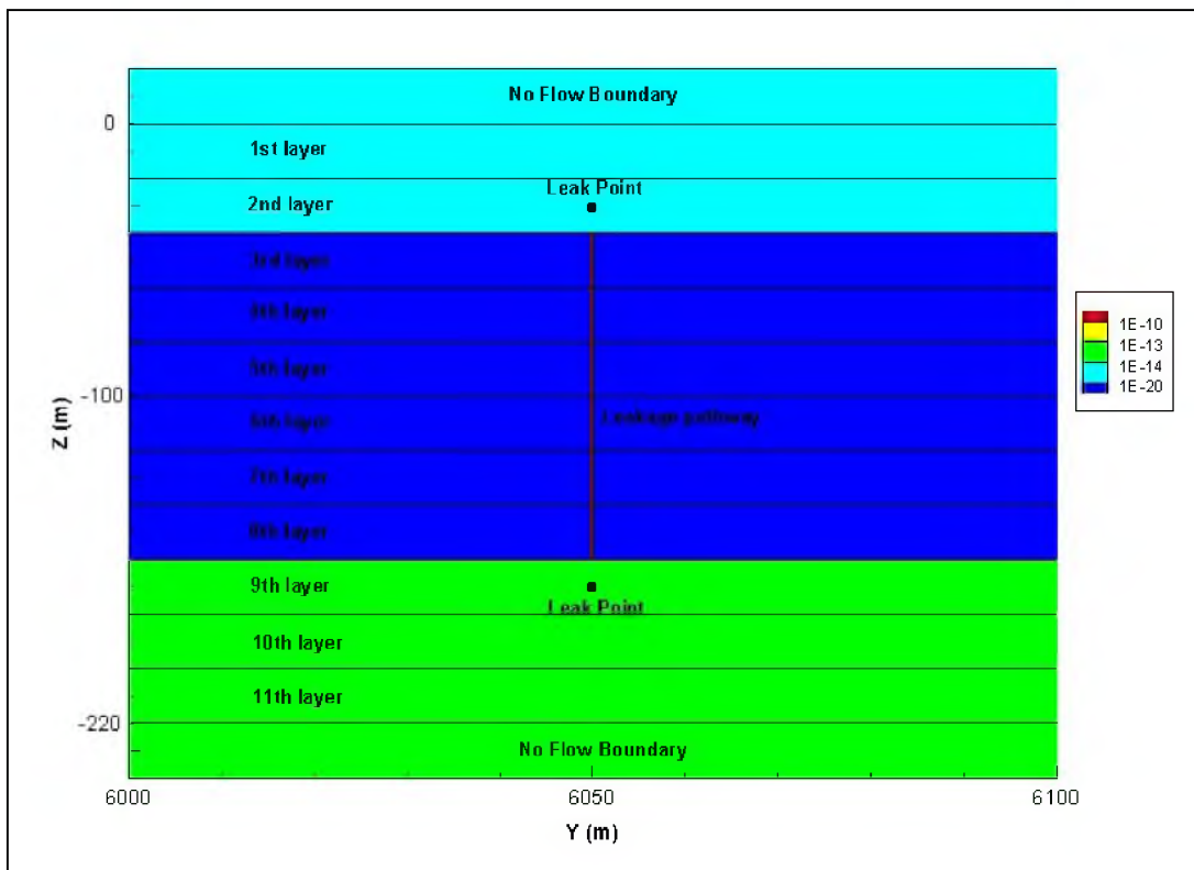
Fig. 5.25 YZ-plane of the leakage pathway in model domain (extended scale).
