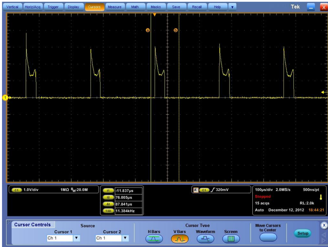
Fig. 4.23. Oscillation waveform of piezoelectric disk based relaxation oscillator.
