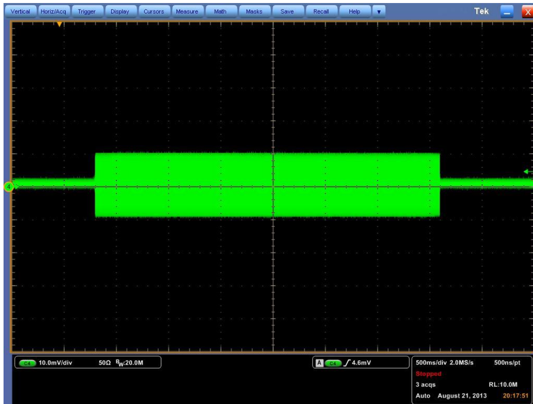
Fig. 6.14. Received oscillation waveforms with frequency modulated by artificial neural signal, to be processed with DSP techniques to restore the neural signal.
