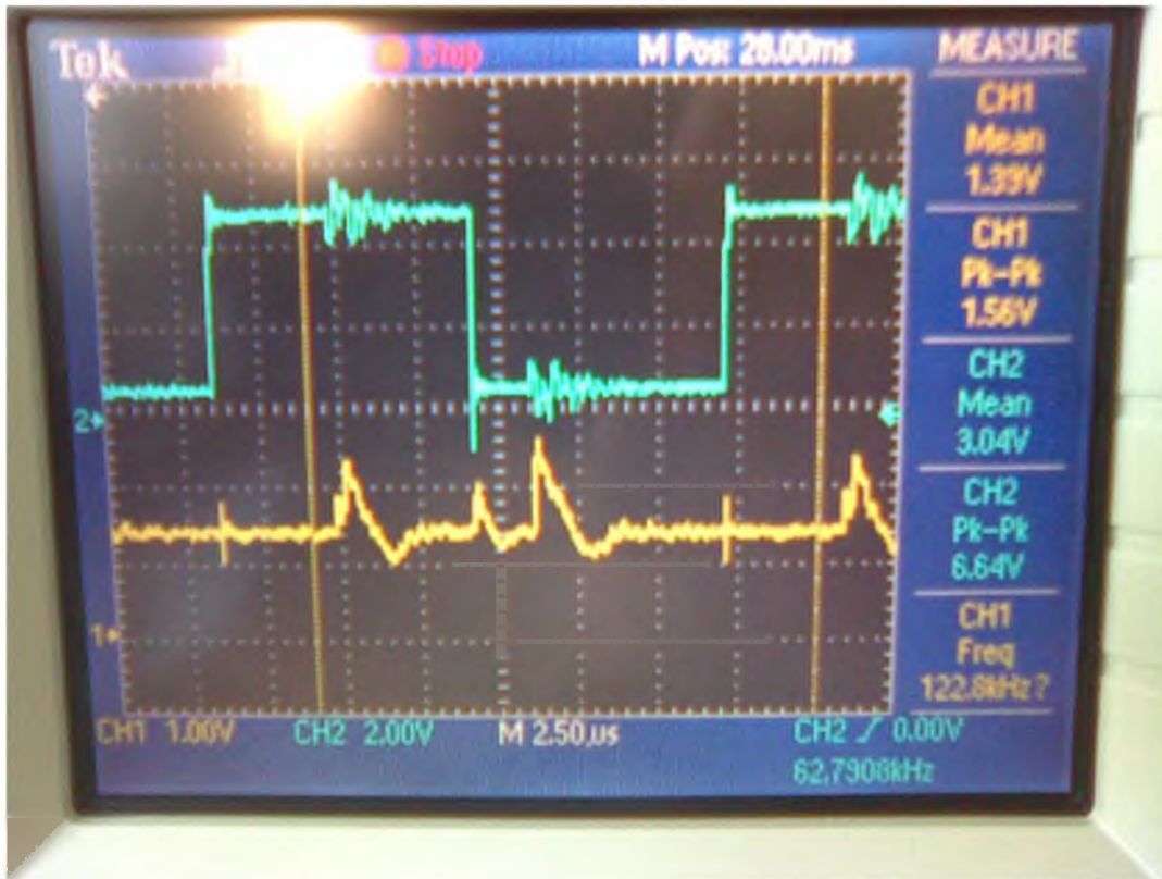
Figure 26: Noise coupled from the PWM signal (blue line) to the load cell signal (yellow line)
