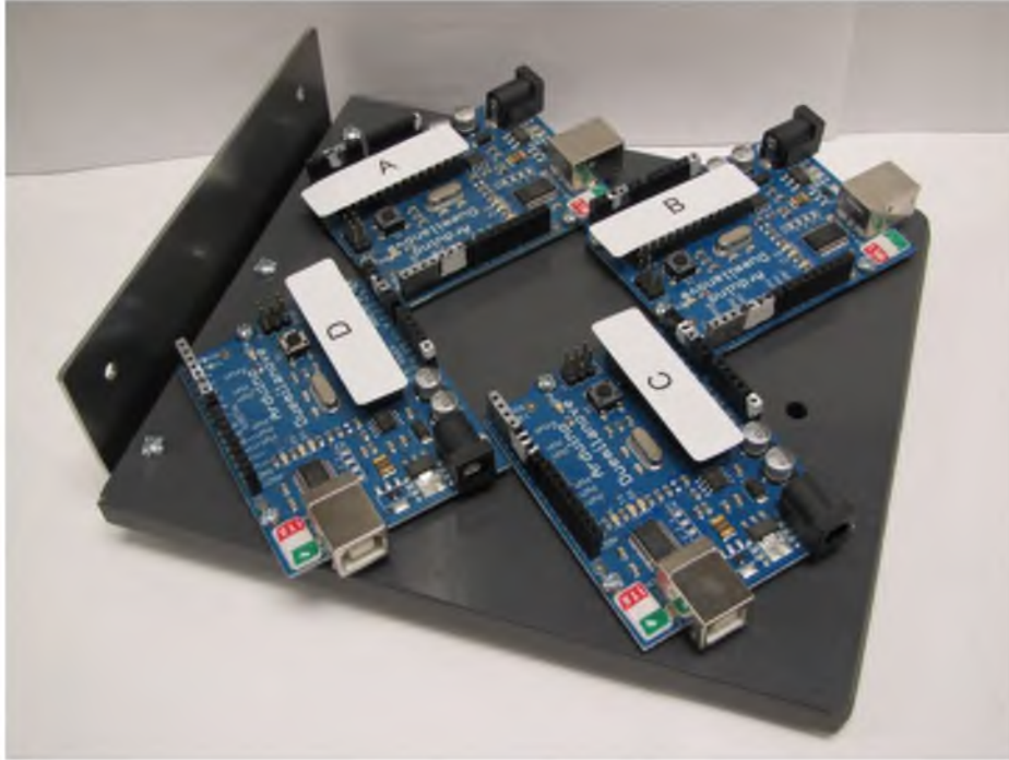
Figure 21: Nonconductive tray for microcontrollers. Note colored pin sockets for correct cable connection/orientation.
