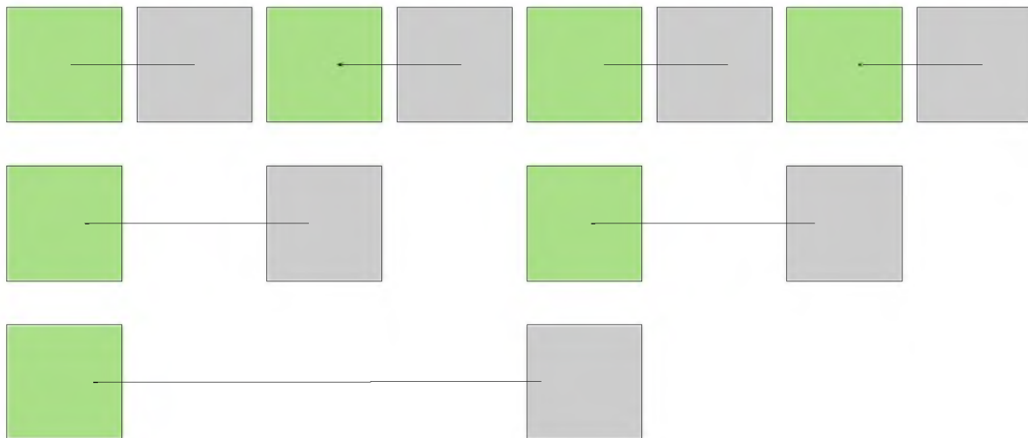
Fig. 2.8. Tree compositing: the green rectangle shows the region each process is authoritative on. The arrows show the direction of the image exchanges. The gray rectangle indicates the region for which the process has data that it is not authoritative on, and will be sending out.
